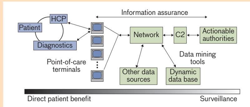
**FIGURE A.** In a system such as that proposed by Lincoln Laboratory in 2002, data mined in various ways are presented to a command and control (C2) center that then informs authorities such as the Centers for Disease Control. Data are fed back to the point-of-care level to aid in diagnosis by health care providers (HCP).
