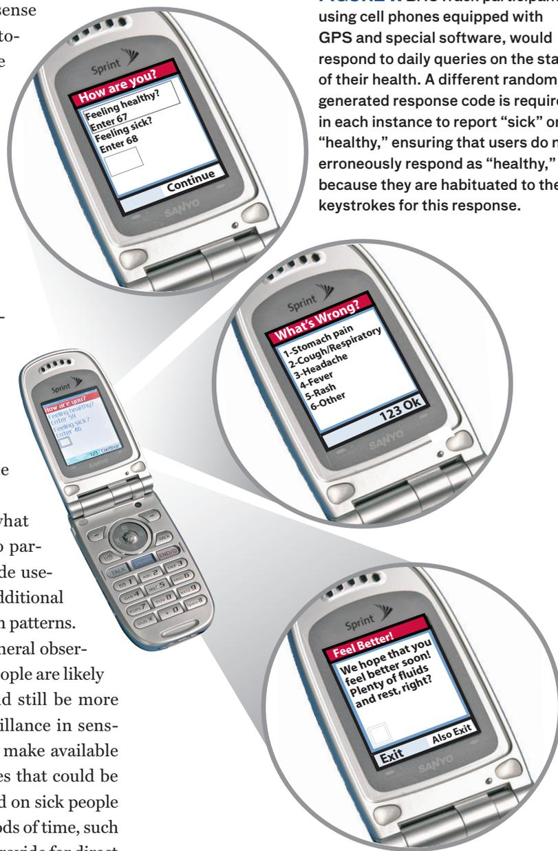
**FIGURE 7.** BACTrack participants, using cell phones equipped with GPS and special software, would respond to daily queries on the state of their health. A different randomly generated response code is required in each instance to report “sick” or “healthy,” ensuring that users do not erroneously respond as “healthy,” because they are habituated to the keystrokes for this response.
