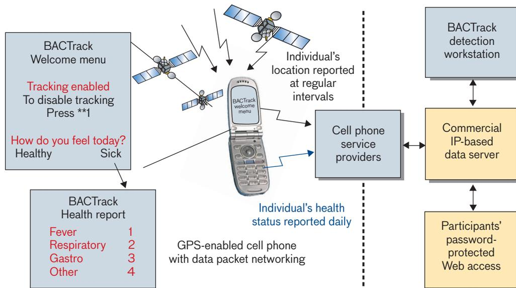
**FIGURE 6.** BACTrack would rely on the GPS technology found in many of today's cell phones. A specialized application would query the volunteer's health status on a regular basis and report back over an Internet Protocol (IP) network to a central analysis server.
