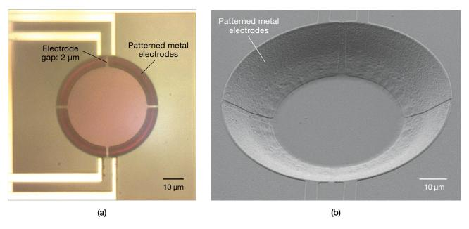
FIGURE 5. The top-down microscope image of the microlens cavity (a) shows the electrode metal deposition and patterning. The scanning electron microscopy image (b) was taken after the microlens was fabricated (the CYTOP film had not yet been applied).
