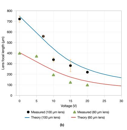
FIGURE 6. In (a), top-down microscope images show the shape of the microlens, which has a diameter of 100  $\mu$ m, at different applied voltages. The graph in (b) plots the focal length versus voltage for fully packaged, planar, single-electrode, liquid microlenses. The microlenses were sealed with deionized water and DC-704 silicone oil.
