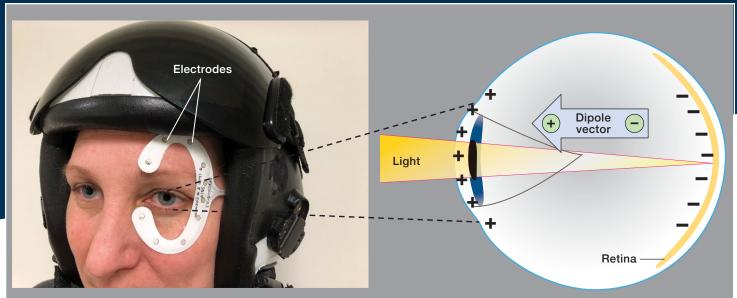
Electrodes detect eye movements by measuring the difference (dipole vector) between the negative electrical charge at the back (retina) and the positive charge at the front of the eye.
