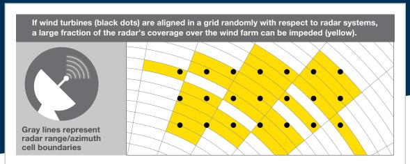
By aligning the wind turbines relative to the radar systems, clear area (white cells) can be opened between wind turbines to restore radar coverage.
