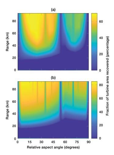
Wind turbines reduce the performance of a radar in a region around them. This graphic shows the percentage of the affected region that is reduced by applying ROWTS as a function of the distance between the radar and wind farm and the relative angle between the radar and prevailing winds, relative to the wind farm. Shown are results from lab-run simulations for (a) a present-day radar and (b) a potential future radar.
