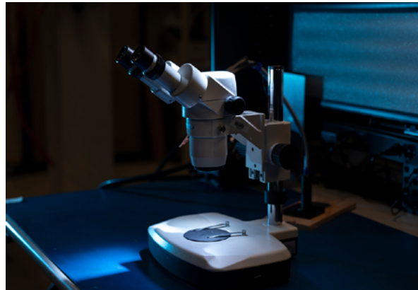
Field microscope used for printed circuit board assembly inspection and repair
