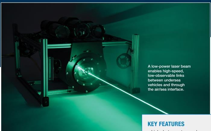
MIT Lincoln Laboratory has developed and demonstrated optical technology for two-way, long-distance communication undersea and through the air/sea interface. This optical system achieves a data rate more than 5,000 faster than today's rates—fast enough to support high-definition video. The system is extremely compact, operates with low power consumption, and is difficult to observe unless directly in the beam path.
