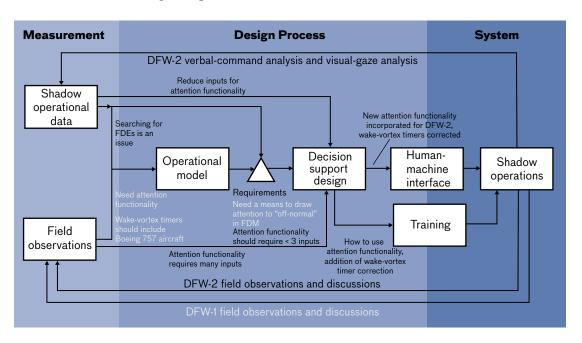
**FIGURE 11.** This TFDM design process model indicates selected requirements and specification modifications made as a result of the DFW-1 and DFW-2 quantitative and qualitative analyses.
