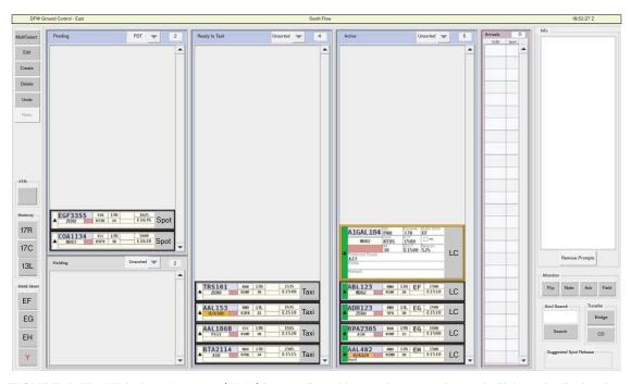
**FIGURE 4.** The Flight Data Manager (FDM) is a configurable, touchscreen, electronic flight-strip display that is interconnected to surveillance information to enable automatic flight-strip movement.
