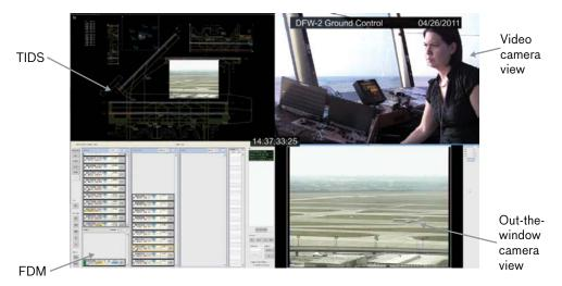
**FIGURE 9.** A video/audio playback system was created for post-demonstration analysis of DFW-2 data. The ability to play back the videos and screenshots simultaneously provided insight into how the controllers used the prototype and aided in identifying which features of the design required further attention.
