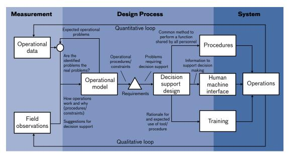
**FIGURE 1.** A benefits-driven, decision support design process provides a means of both qualitatively and quantitatively iterating upon a decision support system (including the human-machine interface, operational procedures, and operational training) to achieve quantifiable operational benefit.
