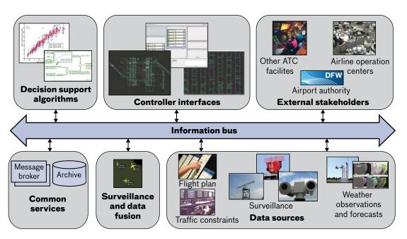
**FIGURE 2.** The Tower Flight Data Manager (TFDM) exhibits a net-centric architecture in which sources such as decision support algorithms publish data to an information bus, while other entities such as controller interfaces subscribe to these data to display to the users.
