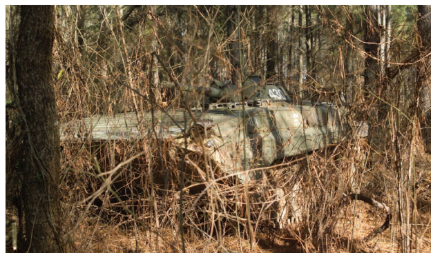
FIGURE 10. Ground vehicles with camouflage and foliage obscurants at the Army Redstone Technical Test Center in Huntsville, Alabama. These vehicles and others were placed in various scenes for 3D imaging tests, including in the clear, within a stand of trees, at the edge of a tree line, and both with and without camouflage net obscurants.
