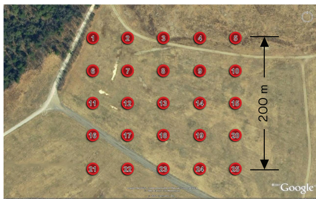
FIGURE 9. The outdoor field tests consisted of 25 sensor nodes arranged on a square grid, spaced 50 m apart. Each node consisted of one battery-powered, tripod-mounted particle counter (either a TSI AeroTrack 8220 or MetOne HHPC-6 EX) and one anemometer (Davis 7911). Wind speed and direction measurements were transmitted in real-time from every sensor node to a base station by using low-power mesh radios (Crossbow Mica2). Sonic anemometers were placed in two locations on the grid for high-fidelity wind data to compare to the Davis 7911 anemometer readings. During the test, 36 smoke candles that produced 40,000 ft 3 of water-based smoke in 30 s were activated. In addition to the concentrations and spread of the 36 smoke releases, measurements of the ambient background were collected periodically throughout the test.
