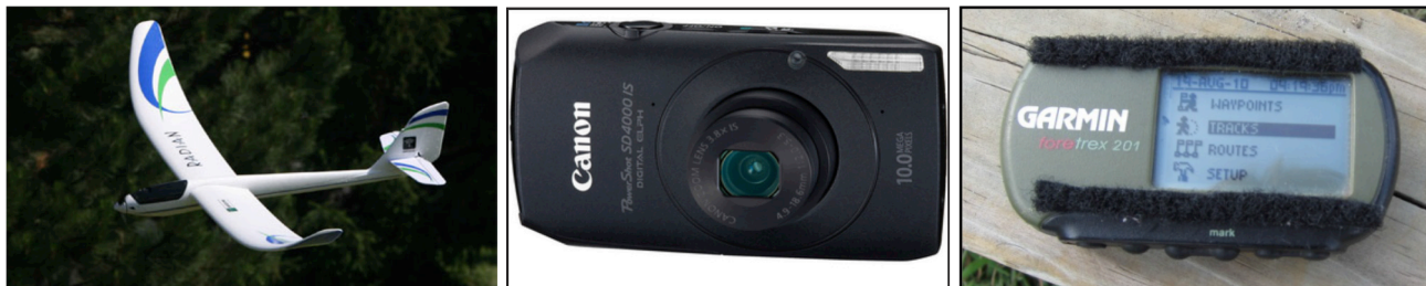
FIGURE 14. Hardware used to collect aerial video over a rural setting included (left to right) a hand-launched sailplane glider, Canon PowerShot camera, and Garmin GPS unit.
