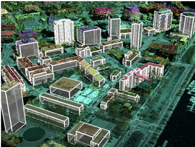
FIGURE 27. Models for 29 buildings around MIT's eastern campus are superposed against the ladar point cloud for Cambridge, Mass.
