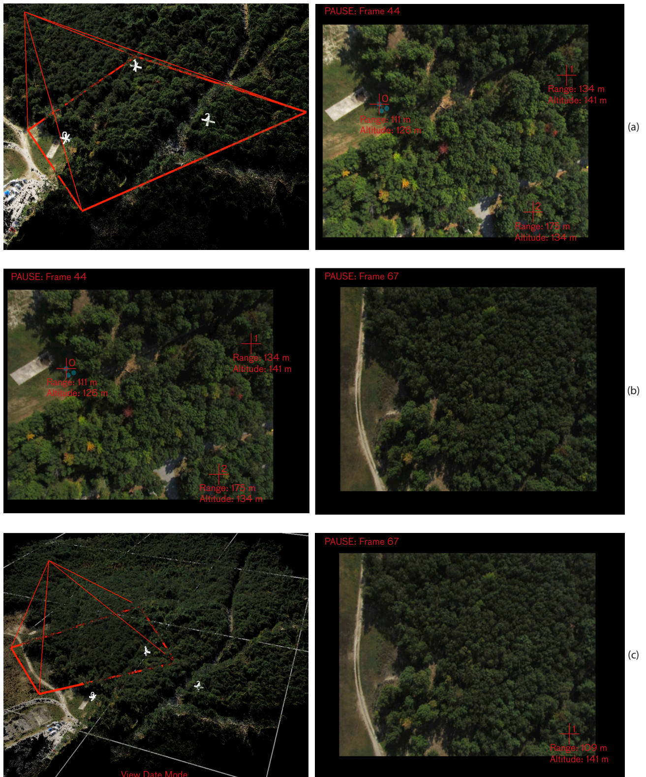
FIGURE 22. (a) 2D pixels selected within the video frame on the right correspond to world-space rays on the left. The selected points are annotated with ranges and altitudes coming from voxels in the dense point cloud that the rays intercept. (b) Determining which, if any, of the pixels selected in the 44th video frame appear in the 67th is difficult for a human eye. (c) Geometry reveals that only pixel 1 in the 44th video frame has a visible counterpart in the 67th frame.
