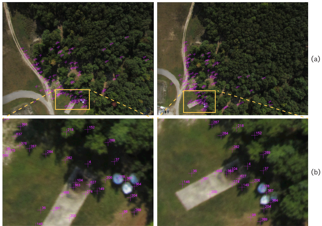
FIGURE 16. (a) 96 SIFT feature matches found between two video frames from the aerial sequence. (b) Zoomed view of tiepoint pairs.
