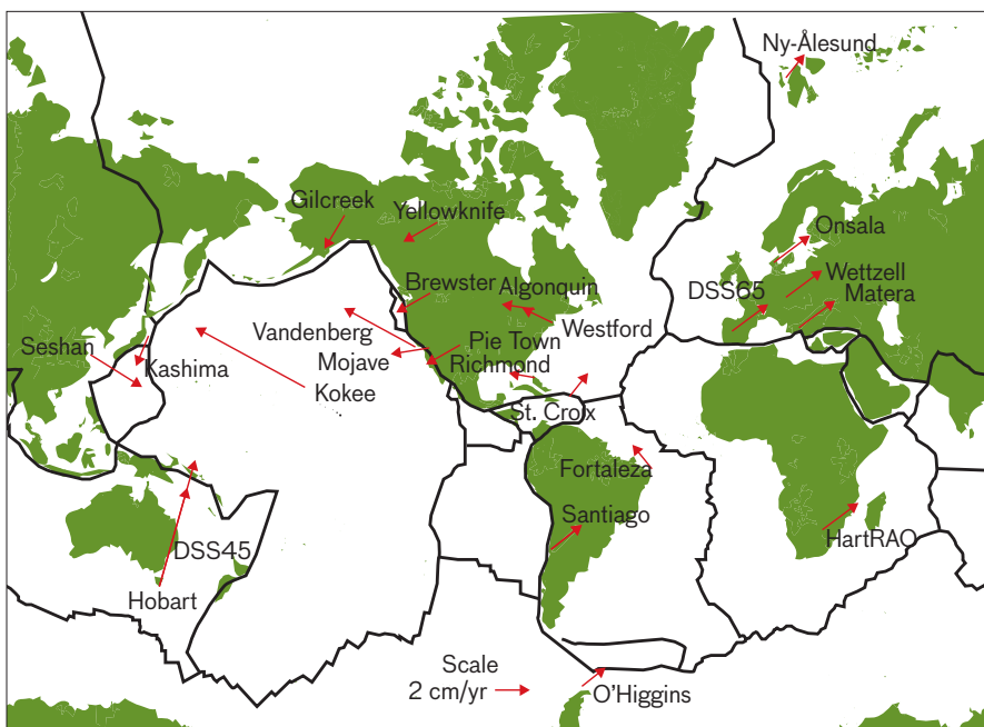
FIGURE 15. Tectonic plate motions were measured with geodetic VLBI; for reference, the Hawaii vector (labeled Kokee) is approximately 8 cm/yr. In this plot, the sum of the tectonic motion vectors is constrained to be zero in order to maintain a net-zero gross rotation rate change. A VLBI antenna is located at the foot of each vector.
