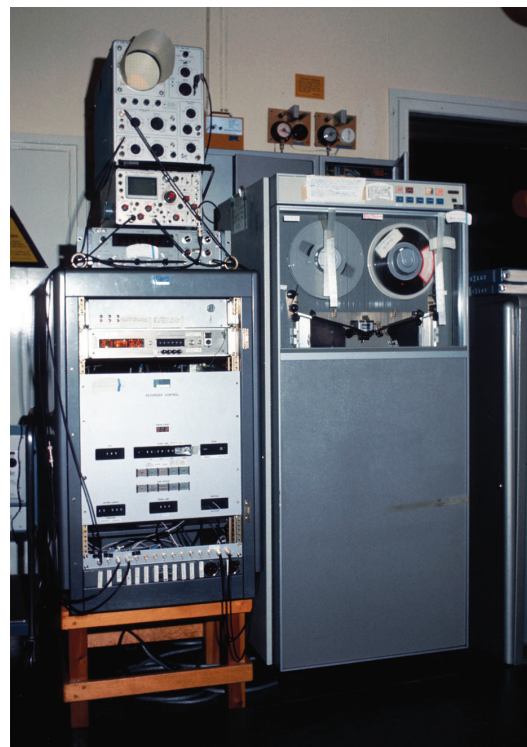
FIGURE 10. The Mark I VLBI recorder captured digitally sampled data at 720 kbps onto a standard 12-inch computer tape that filled in 3 minutes.
