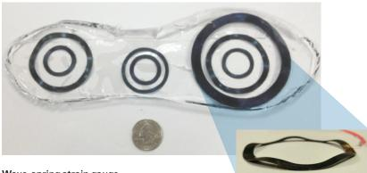
Wave-spring strain gauge.
