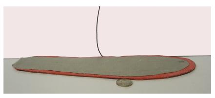
Capacitive load-sensor insole with readout electronics.
