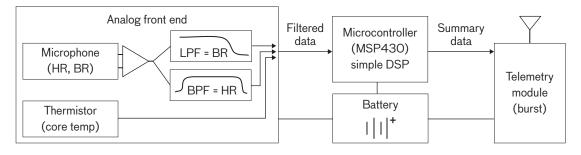
Schematic of an ingestible electronic device that concurrently measures heart rate (HR), breathing rate (BR), and core temperature (CT). Acoustic signals recorded from the microphone are fed through a low-pass filter (LPF) and band-pass filter (BPF) and then sent to a microcontroller that performs simple digital-signal processing (DSP) to determine HR and BR.
