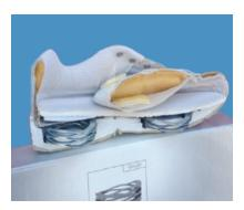
Wave-washer strain gauge insert (wave washer in inset).
