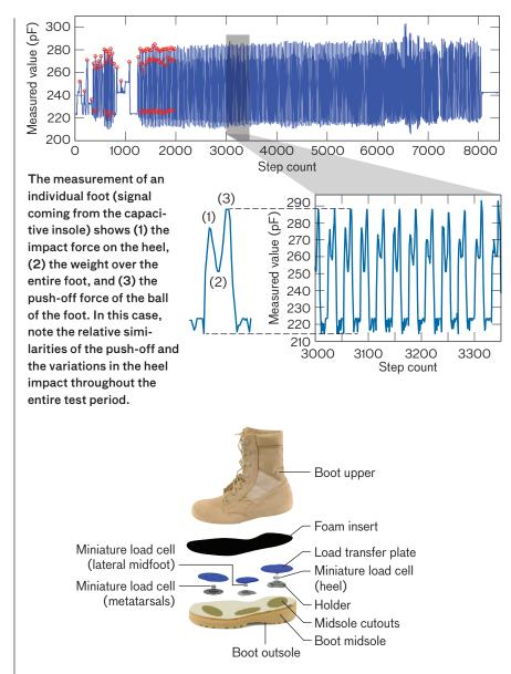
Load cells, positioned at three discrete points on the foot, are integrated into the midsole of a standard warfighter boot.
