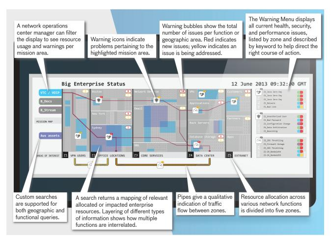
Annotated display of computer network operations explains design functionalities that facilitate situational awareness. By consulting the Warning Menu on the right-hand panel, a network operator will note, for example, that in Zone 1, there is a bad link (color-coded in blue) that is being addressed (yellow).
