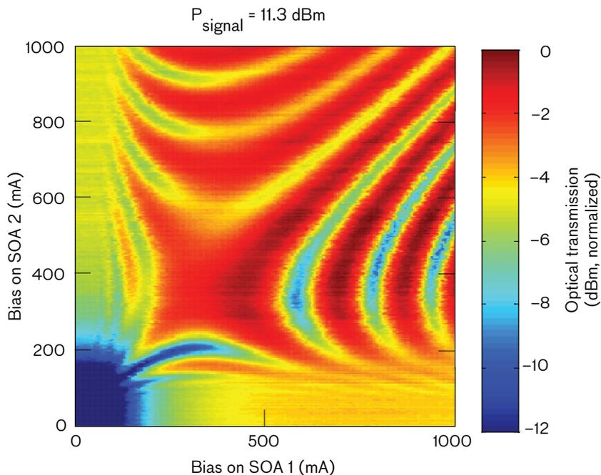
The color-coded map shows constructive and destructive interference as a function of bias current on the two semiconductor optical amplifiers (SOA 1 and SOA 2). Constructive interference between the two interfering light beams, shown in deep red, results in high optical transmission (a digital 1), while destructive interference, shown in blue, produces low optical transmission (a digital 0).
