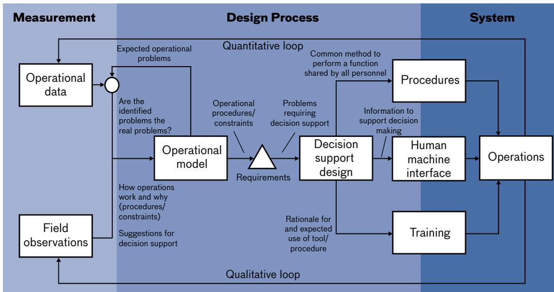
**FIGURE 1.** A benefits-driven, decision support design process provides a means of both qualitatively and quantitatively iterating upon a decision support system (including the human-machine interface, operational procedures, and operational training) to achieve quantifiable operational benefit.
