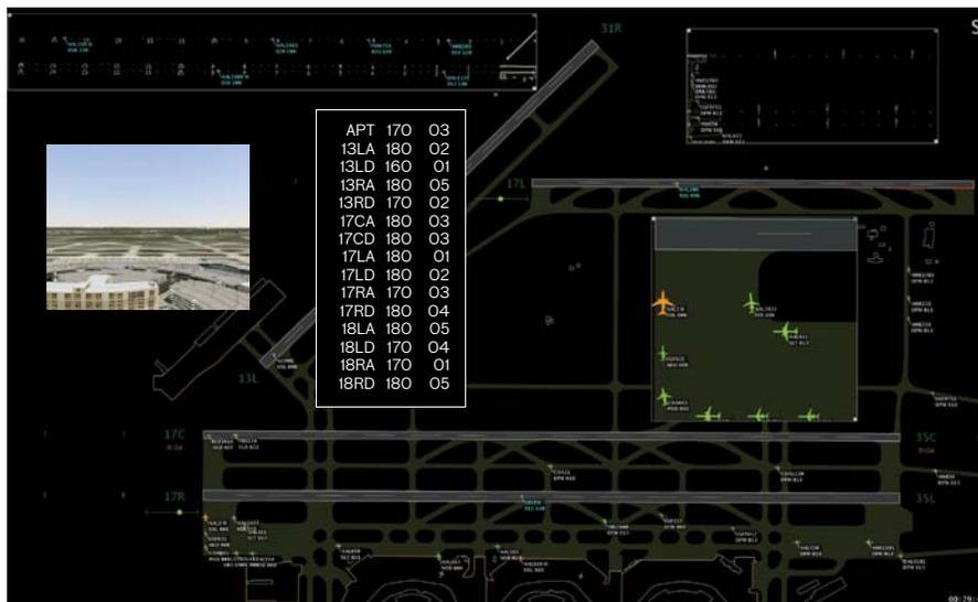
**FIGURE 3.** The Tower Information Display System (TIDS) is an advanced surveillance display that contains surveillance processing enhancements over the current ASDE-X surveillance display as well as interface improvements.
