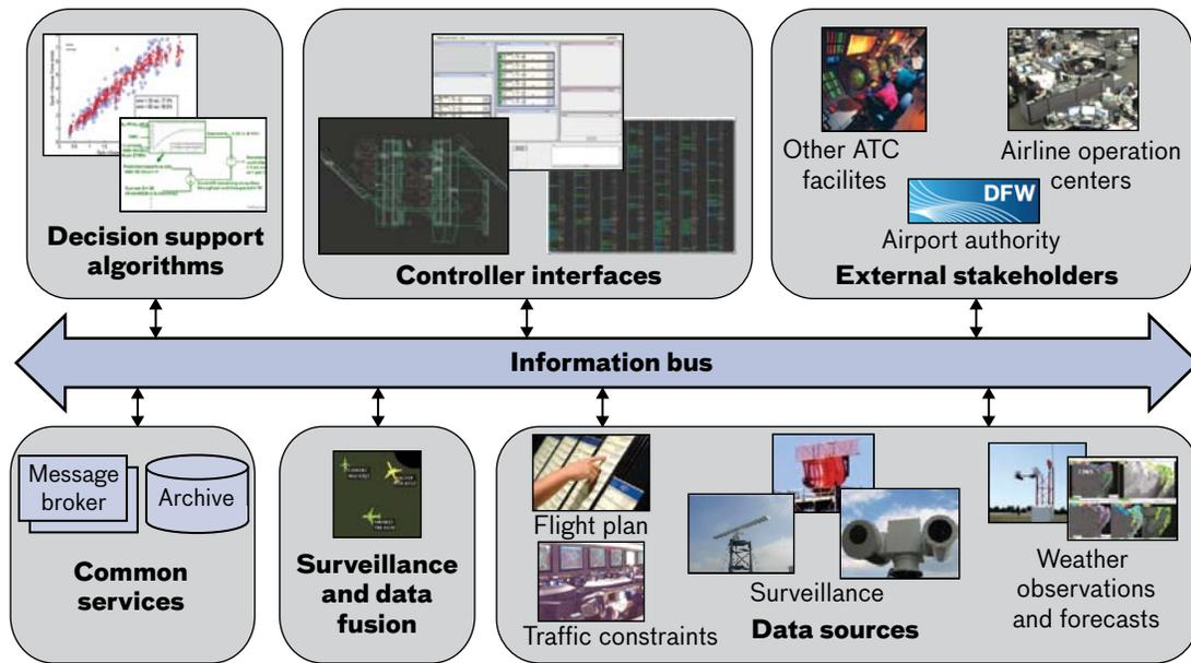
**FIGURE 2.** The Tower Flight Data Manager (TFDM) exhibits a net-centric architecture in which sources such as decision support algorithms publish data to an information bus, while other entities such as controller interfaces subscribe to these data to display to the users.
