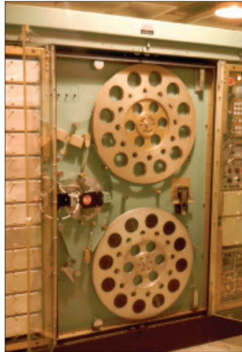
**FIGURE 5.** The early TRADEX radar saved its data on this analog intermediate-frequency tape recorder.
