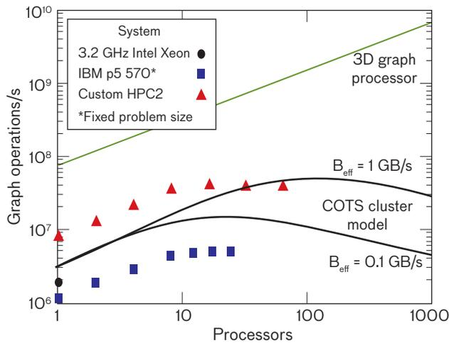
**FIGURE 14.** The computational throughput performance projections were made based on simulations. The 3D graph processor achieved orders of magnitude better computation performance than the commercial systems.
