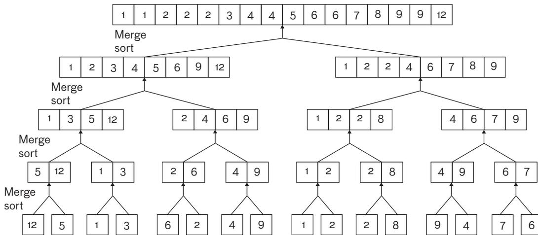
**FIGURE 7.** In this conventional 2-way merge sort, 16 items are sorted in four steps.
