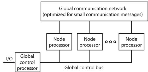
**FIGURE 4.** The illustration of the high-level architecture for Lincoln Laboratory’s parallel graph processor shows the connection between the specialized sparse matrix processors (node processors) and the global components.
