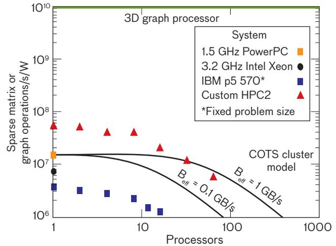
**FIGURE 15.** Power efficiency projections versus number of parallel processors were made based on simulations. The power-efficiency difference compared to commercial processors is expected to be even larger than the computational throughput difference as the number of processors grows because the computational throughput does not level off as in commercial processors.
