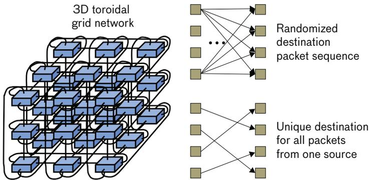
**FIGURE 13.** This illustration of the 3D graph processor with electromagnetic coupling communications between processor boards shows the contrast between a randomized destination and a unique destination in a simulation using a 512-node 3D toroidal network. In the randomized destination case, 87% full network efficiency is achieved. In the unique destination case, only 15% full network efficiency is achieved.
