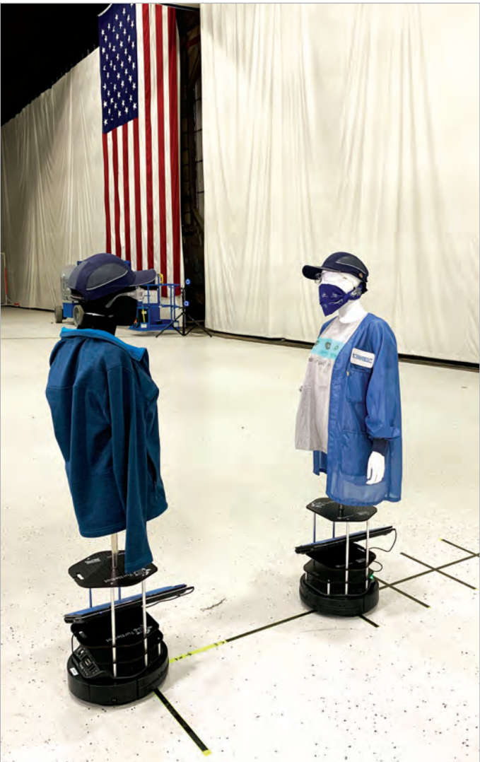
In the Autonomous Systems Development Facility, Laboratory researchers use robots to test the Private Automated Contact Tracing (PACT) mobile application and its ability to detect close, prolonged contact via Bluetooth with another PACT-enabled device. If a PACT user tests positive for COVID-19, that person can enable the app to alert other users of possible exposure, without revealing any personal information.
