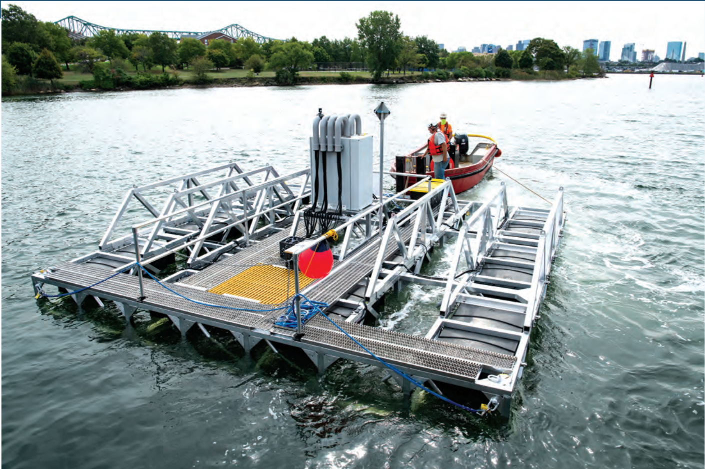
Researchers deployed a technology demonstrator of an undersea mapping sparse sonar array. The array is a novel surface-based, distributed multi-input multi-output sparse aperture sonar to support deep ocean floor mapping with a resolution two orders of magnitude higher than is currently achievable.
