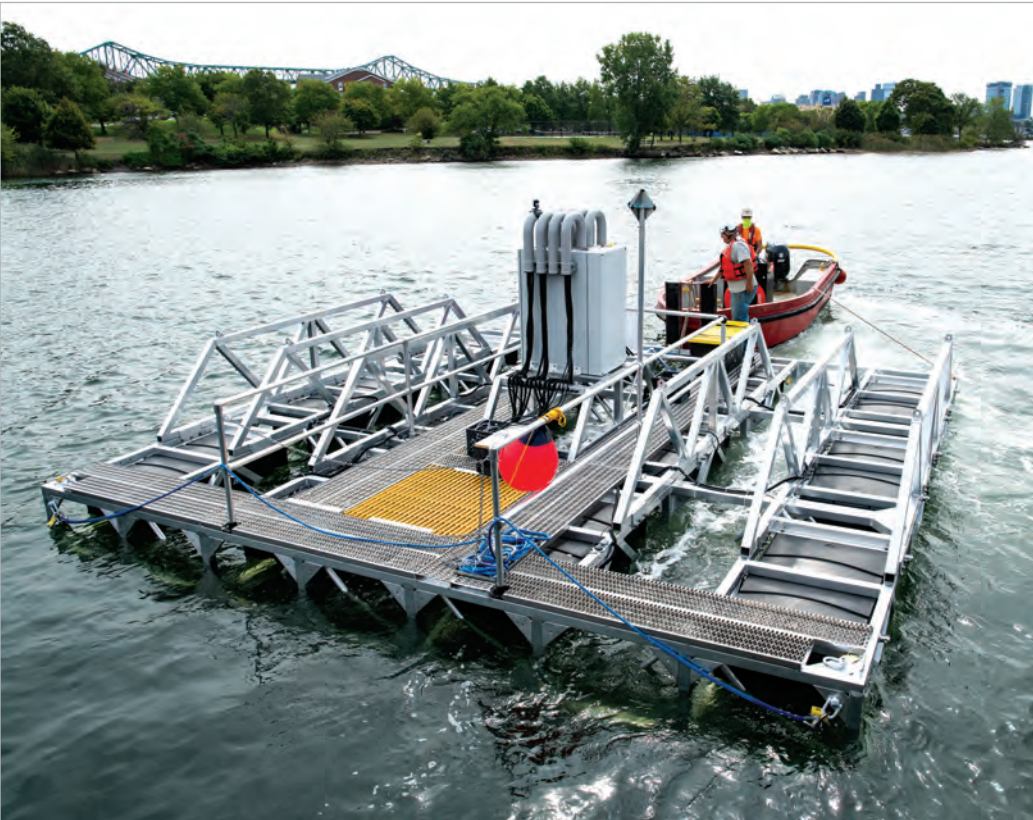
Researchers deployed the technology demonstrator of an undersea mapping sparse sonar array. This array (24 × 24 feet) is a surface-based, distributed multiple-input, multiple-output sparse aperture sonar designed to support deep ocean floor mapping with a resolution two orders of magnitude greater than what is currently achievable.
