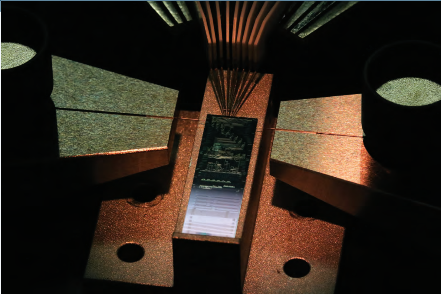
Photonic integrated circuit (PIC) optical matched filters achieved excellent filter extinction (>45 dB) and highly Gaussian lineshape. Coupled with advanced digital signal processing, PIC technology will dramatically reduce the size, weight, power, and cost of future lasercom terminals.
