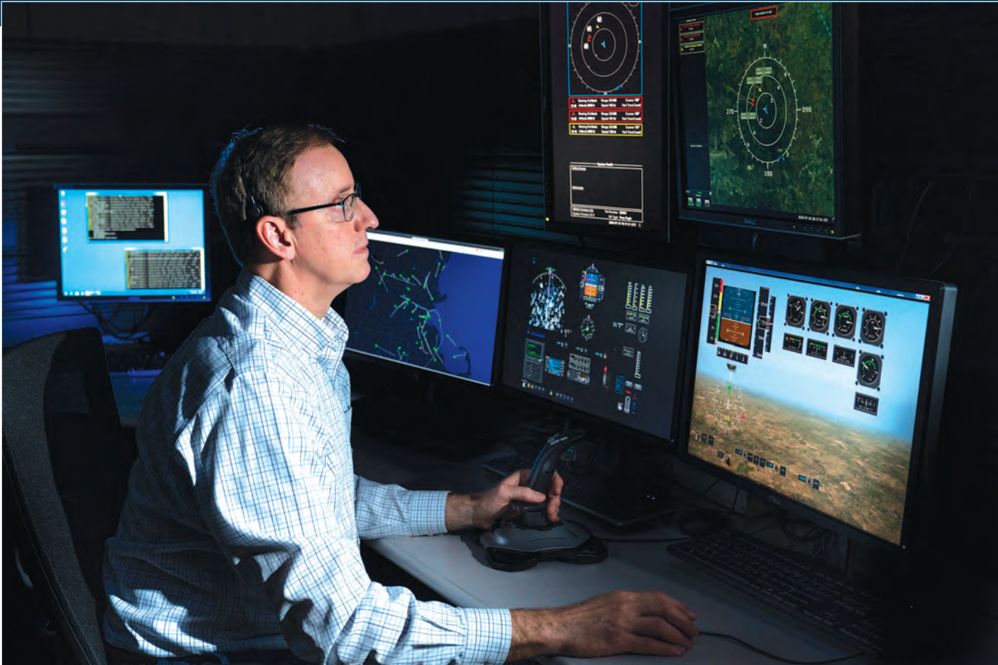
The Laboratory's Ground-Based Sense and Avoid system, operational at 12 military installations, provides maneuvering guidance to unmanned aircraft system operators to help them avoid nearby aircraft.
