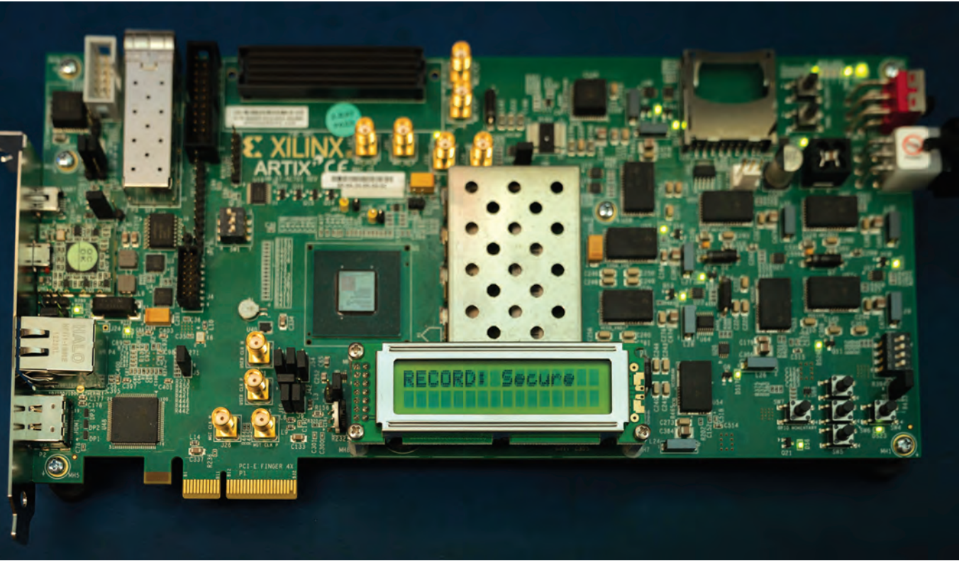
Shown is a prototype of RECORD (Reconfigurable Edge Computing for Optimum Resource Distribution), a low-power self-reconfigurable processor that adapts its resources to minimize power consumption while securing the system during configuration and operation. RECORD is intended for deployment in environments where secure, long-endurance unattended computational capabilities are needed, such as remote monitoring systems.
