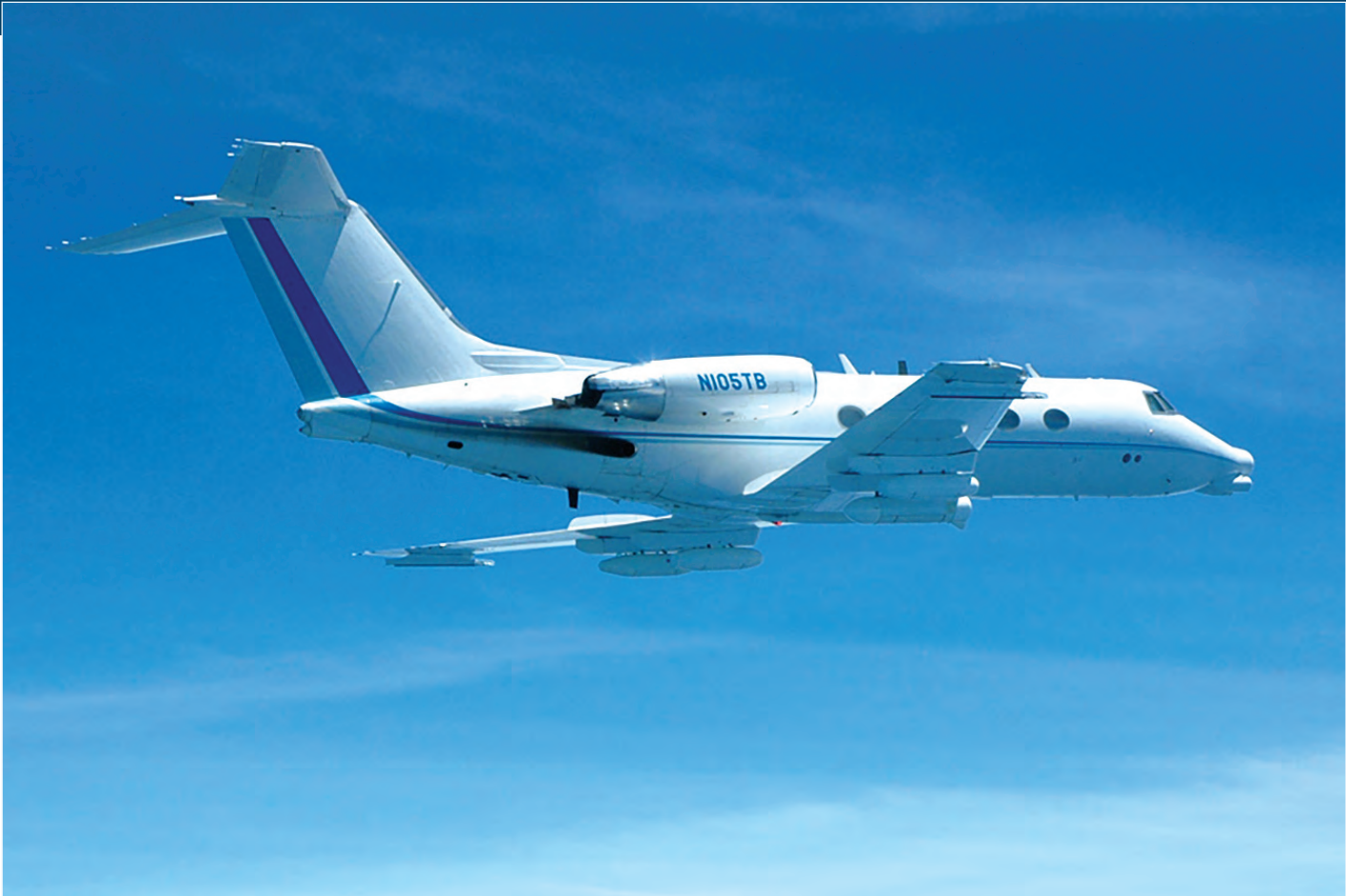
The Airborne Seeker Test Bed is a customized aircraft used in flight testing radio-frequency and infrared sensors. To carry these sensors, the aircraft is modified with wing pylons, a nose radome, forward chin-pods, and computer and instrumentation racks in the interior.
