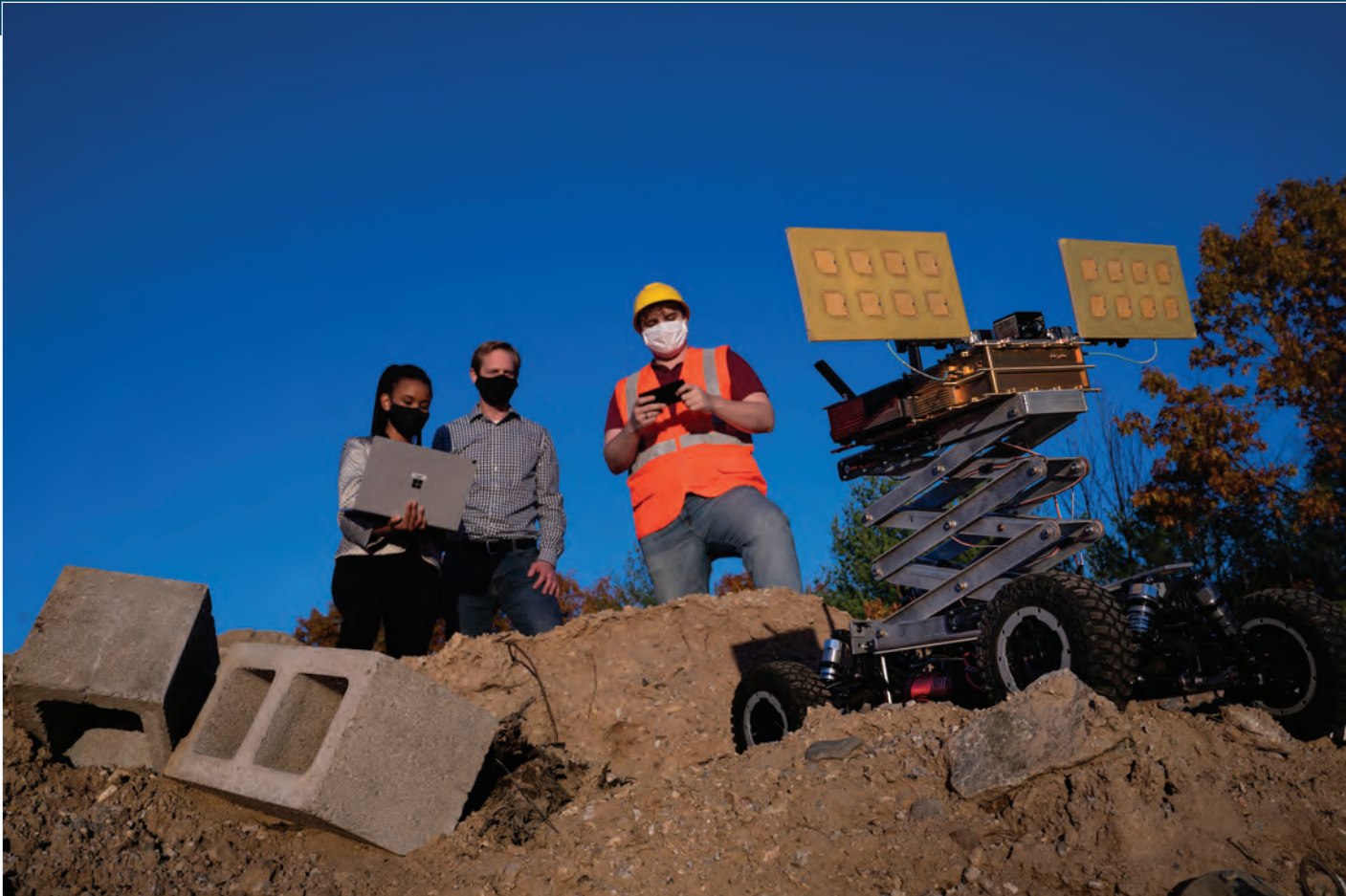
A radar system integrated on an unmanned ground vehicle can detect disaster survivors trapped under rubble. The radar extracts a breathing rate and wirelessly transmits the data and the location to rescue teams. Future work will focus on unmanned air vehicle integration.
