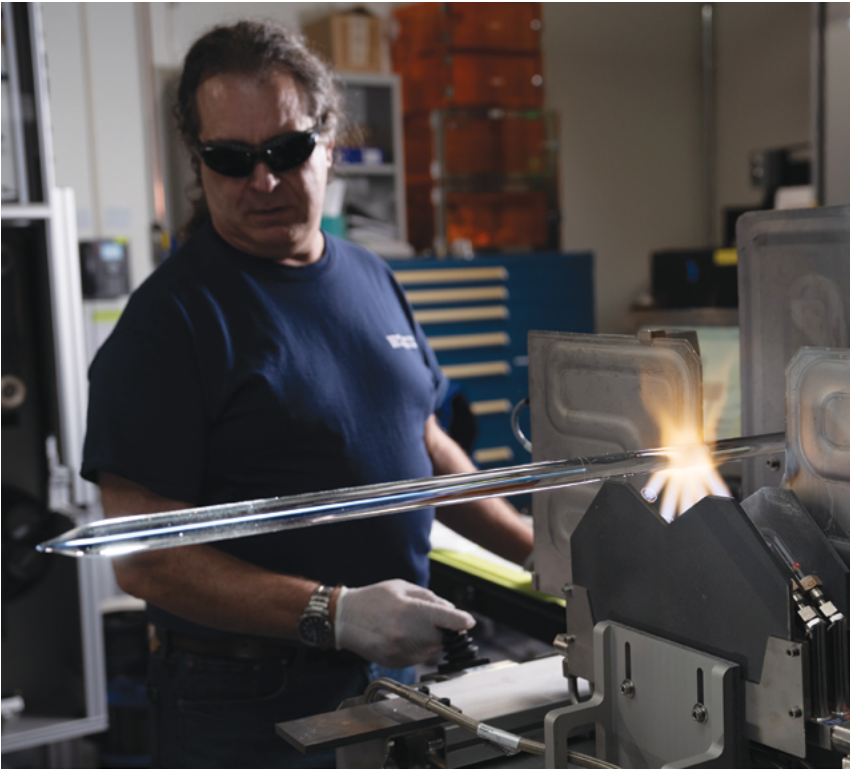
Rich Molnar flame-polishes a silica-rod preform before it is drawn into optical fiber. The draw process will change the form of the rod to a submillimeter fiber stretching kilometers in length. Rare-earth elements such as ytterbium can be added into the core of the fiber to act as lasing centers. Other engineered glasses, such as aluminophosphate glass developed through this Technology Office program, are used to guide light down the fiber.
