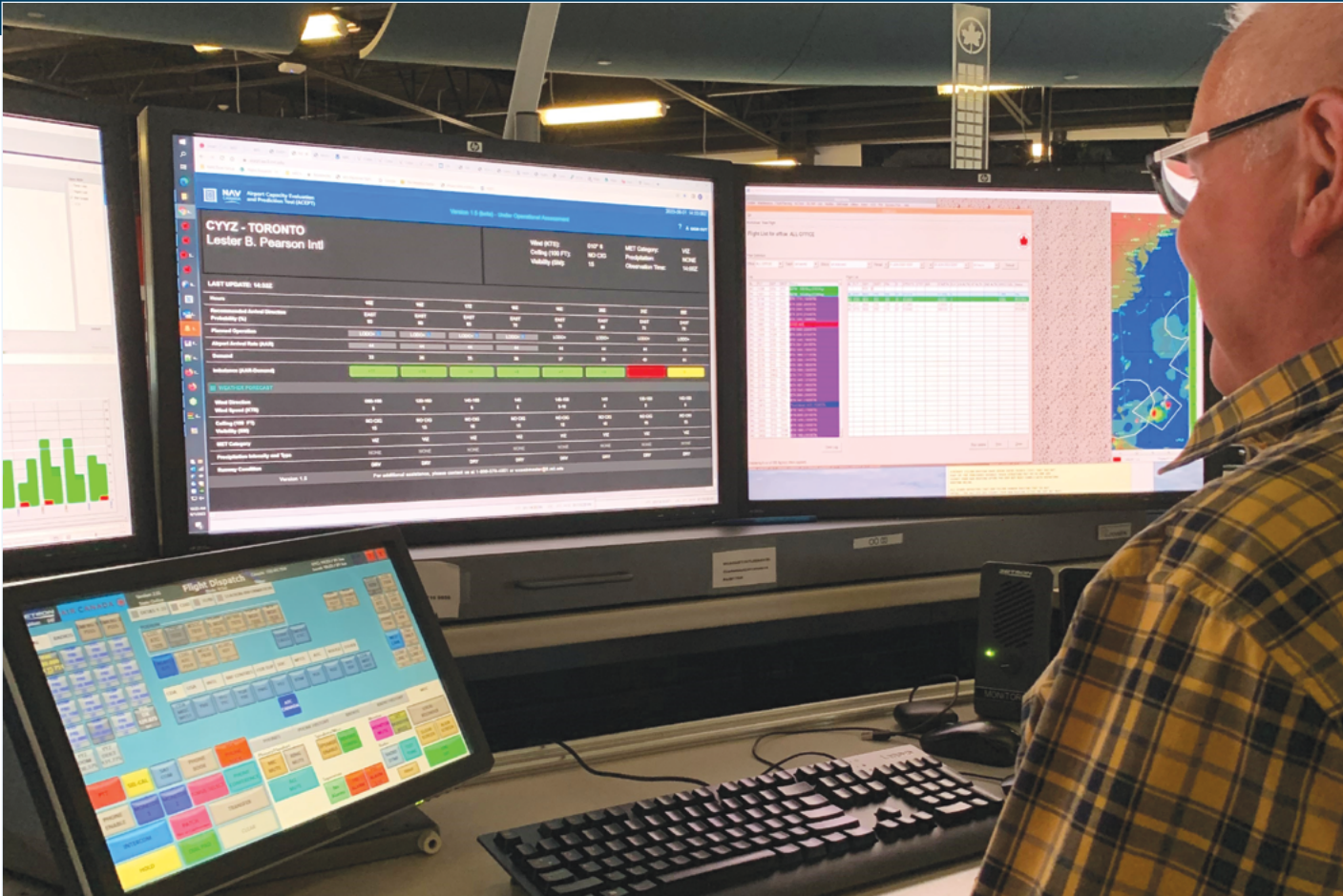
Lincoln Laboratory collaborated with NAV CANADA to develop integrated technologies for predicting the impact of weather on aviation. Here, an airline dispatcher uses the Laboratory's Airport Capacity Evaluation and Prediction Tool to assess capacity and demand at Toronto Pearson Airport.
