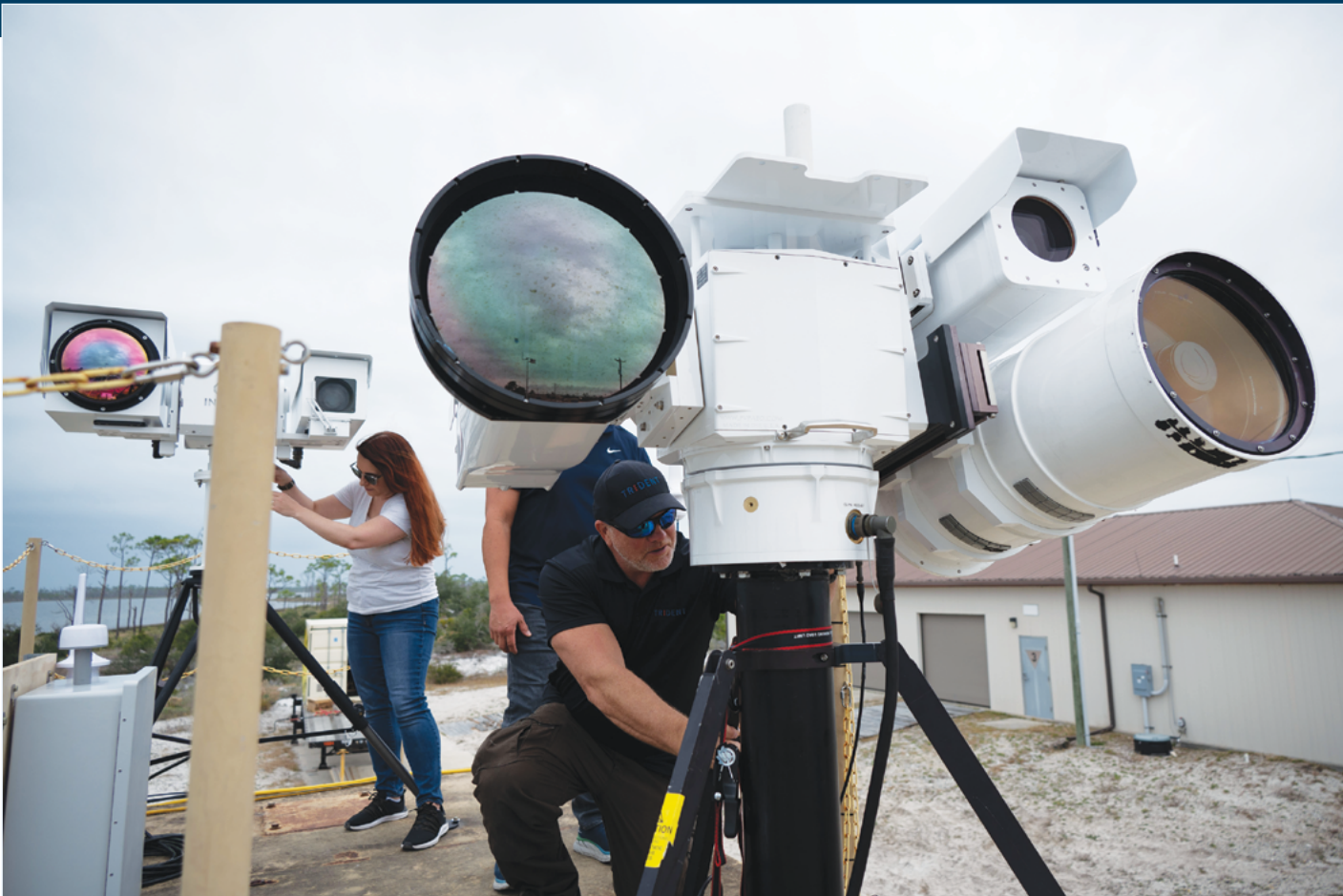
Lincoln Laboratory developed a test bed at Ramstein Air Base in Germany for evaluating air defense sensors, software, and decision support tools. This test bed was downsized for an exercise in Florida, where team members, above, deployed sensors identical to those tested in Germany.
