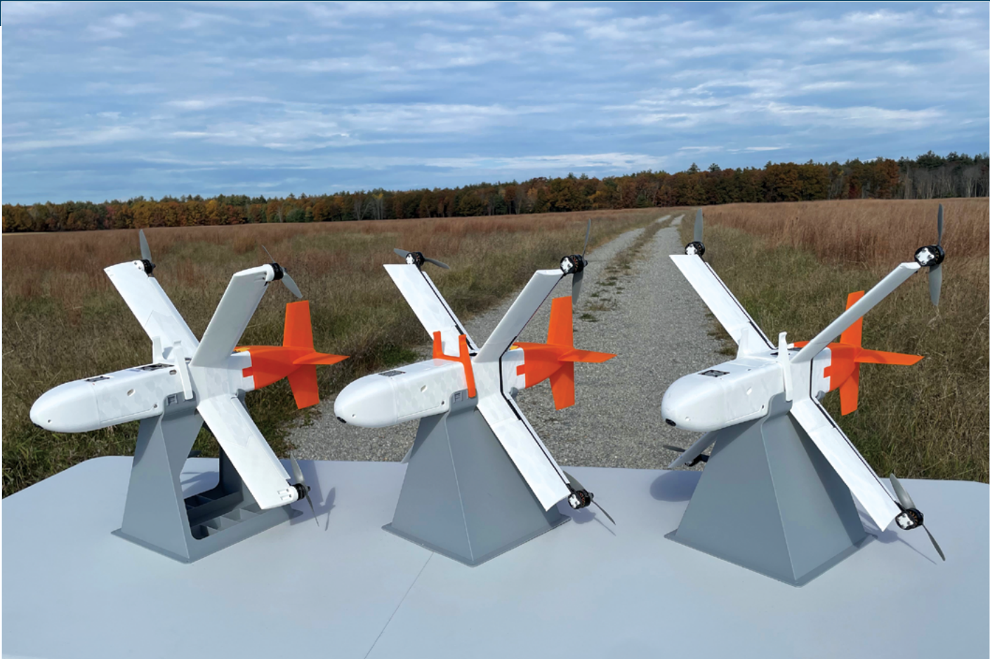
The Small Inexpensive Counter Air (SICA) program demonstrated drone capabilities at an event hosted by the DoD. Each SICA drone, shown above, is estimated to cost less than $7,000 and uses a Laboratory-developed low-cost sensor to provide defense against one-way attack drones.
