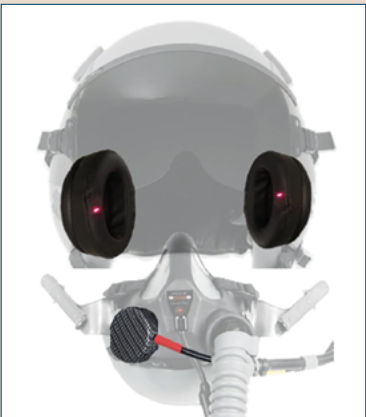
Spotlight Lab's SPYDR sensor suite, incorporated into a pilot's helmet, gathered data for demonstrations of the algorithms that calculate physiological state.
