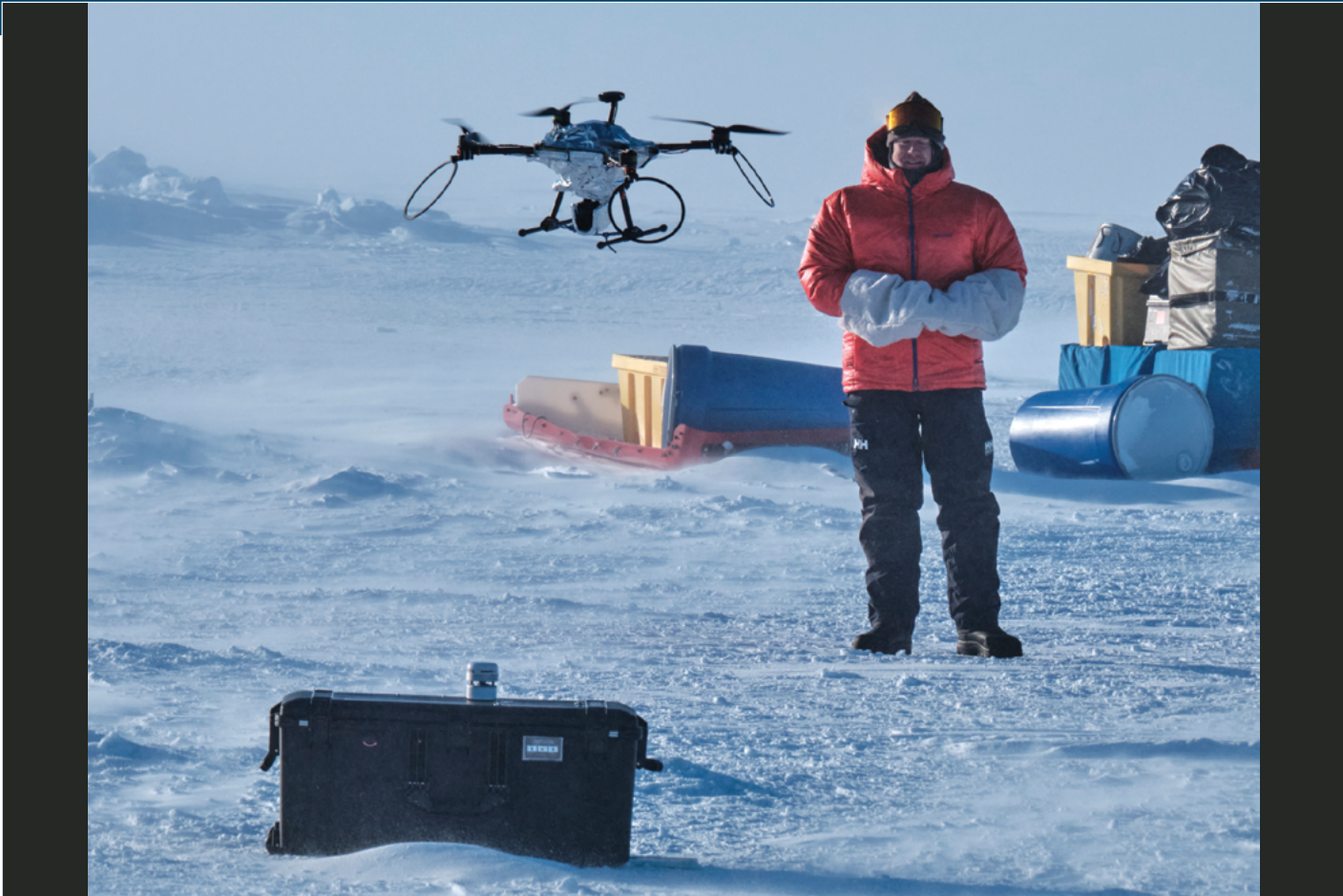
David Whelihan flies a drone to retrieve data from a Laboratory-developed integrated sensor node deployed in the Arctic during Operation Ice Camp 2024. The node is intended to become part of a widespread sea-ice monitoring network.
