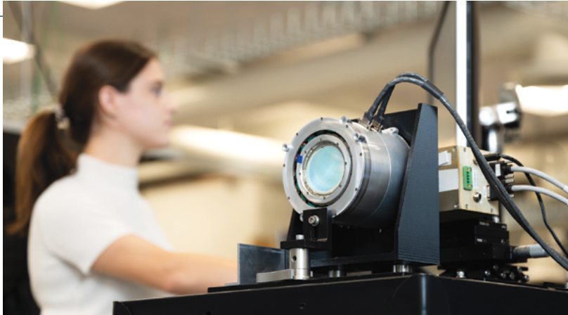
Emma Chadwick operates a prototype optical system consisting of a novel scanner paired with an advanced camera capable of digital processing at the pixel level. This combination potentially enables rapid wide-area scanning in a compact form factor that could fit on small satellites for global surveillance applications. Current laboratory testing is focused on characterizing system performance and developing key image-processing algorithms.
