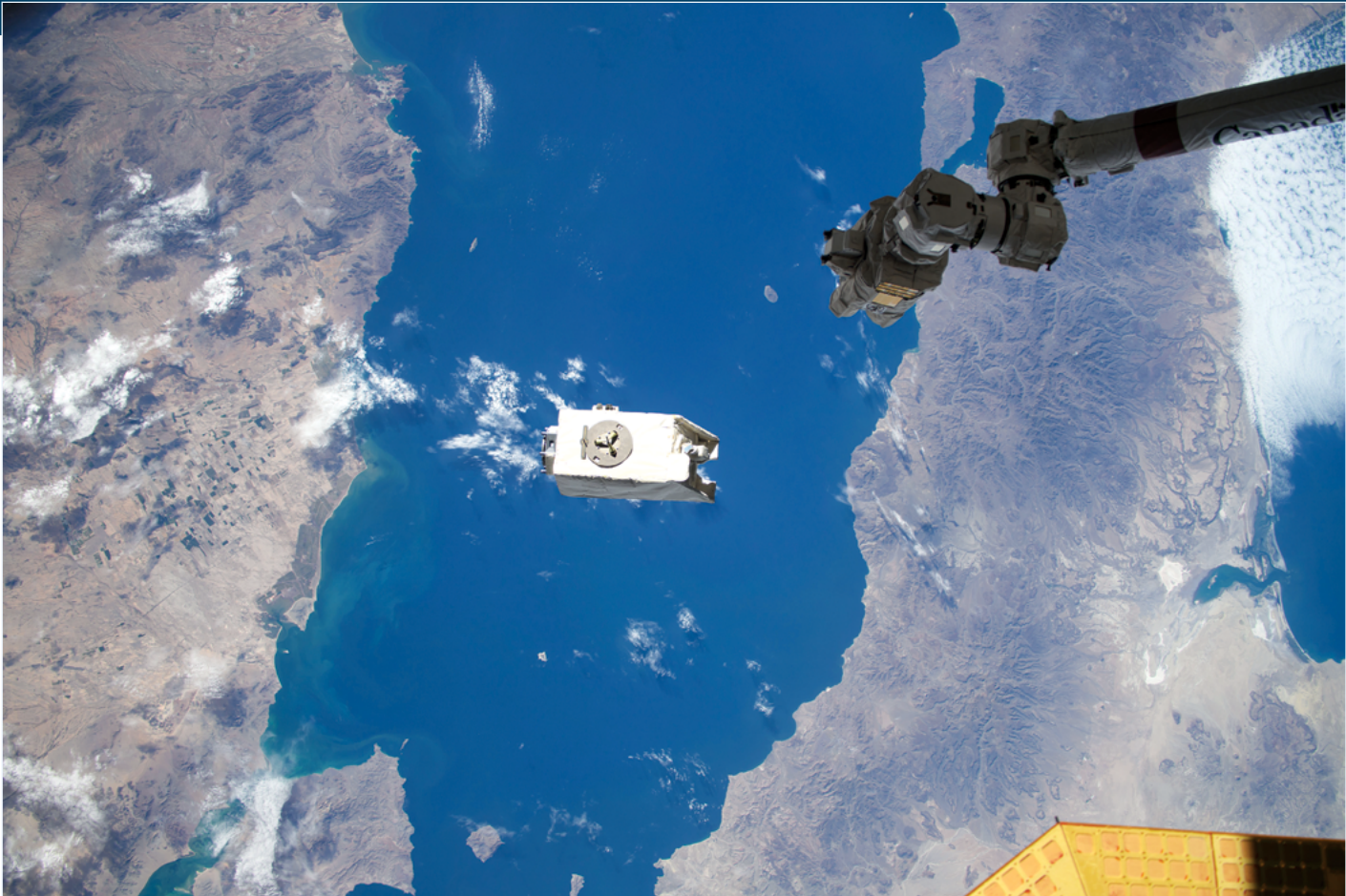
The Laboratory’s Integrated Lasercom Relay Demonstration (LCRD) Low Earth Orbit User Modem and Amplifier Terminal (ILLUMA-T) released from the International Space Station in June 2024 after six months of testing. ILLUMA-T and LCRD demonstrated NASA’s first in-space two-way lasercom relay.
