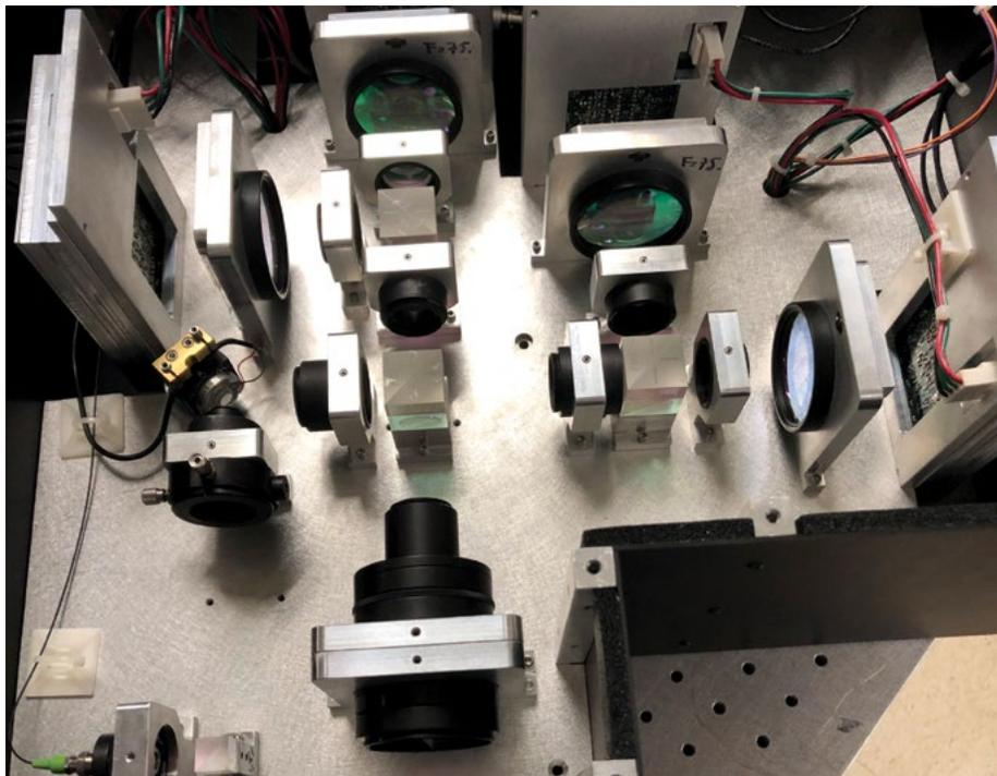
**FIGURE 11.** The skin- and eye-safe laser Doppler vibrometer utilizes 48 pixels simultaneously. The system has a bandwidth of 5 megahertz and uses 2-inch collection optics that can be operated from a stand-off distance of 100 to 500 millimeters. The laser has an output of 10 milliwatts and an adjustable manual focus.
