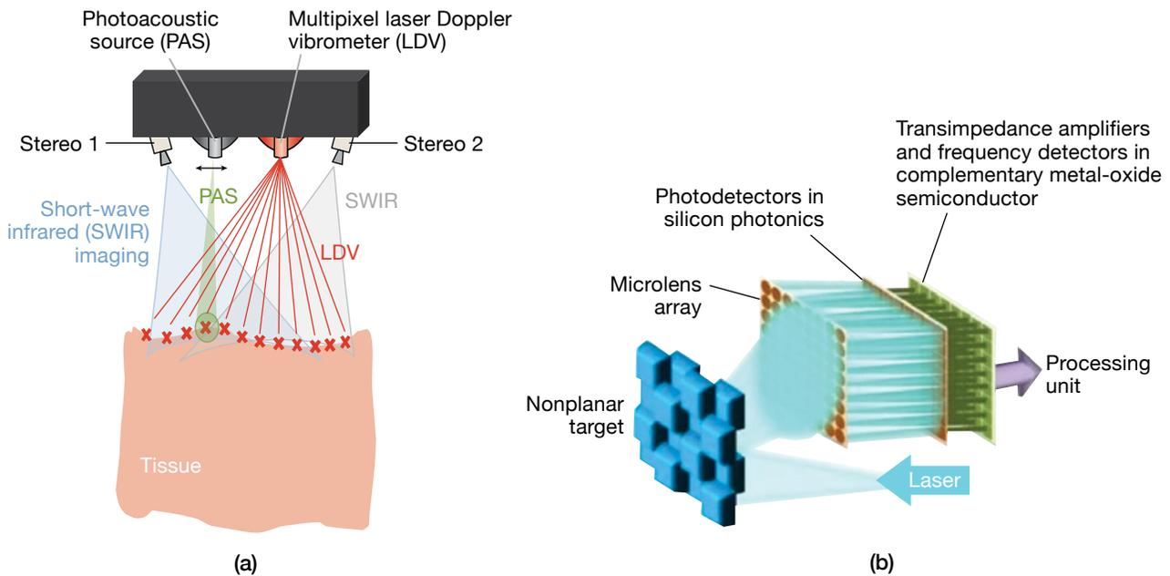
**FIGURE 13.** A portable handheld N-CLUS system concept is illustrated (a). The system would contain a photoacoustic source and a laser Doppler vibrometer on the same unit. Coherent focal plane arrays (b) are being considered as an element to integrate into medical ultrasound, but significant development is needed to implement chip-scale lidar and coherent focal plane array technology on medical devices.
