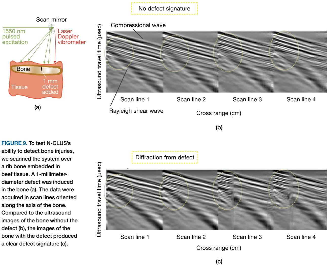
**FIGURE 9.** To test N-CLUS’s ability to detect bone injuries, we scanned the system over a rib bone embedded in beef tissue. A 1-millimeter-diameter defect was induced in the bone (a). The data were acquired in scan lines oriented along the axis of the bone. Compared to the ultrasound images of the bone without the defect (b), the images of the bone with the defect produced a clear defect signature (c).
