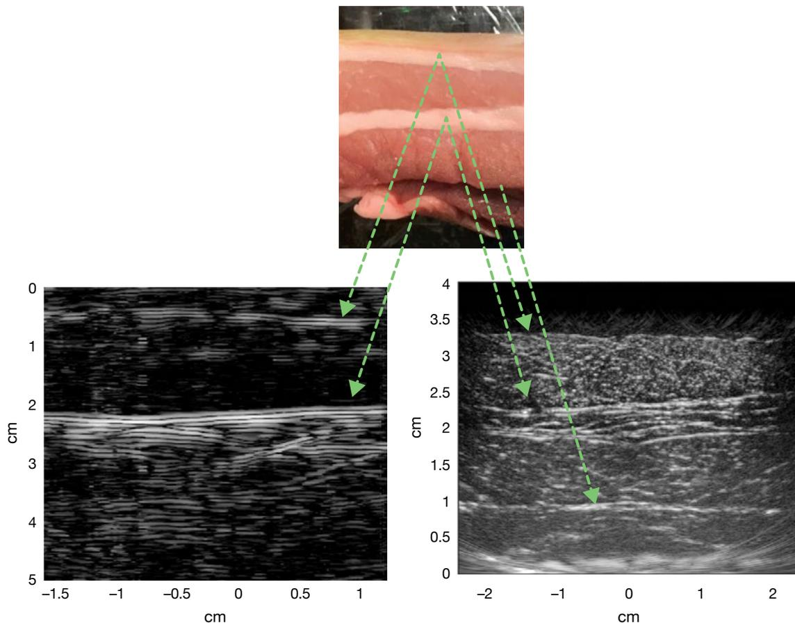
**FIGURE 6.** The above figure shows the N-CLUS sonograms of a scanned pork sample, converted to depth. Comparisons are shown for the total N-CLUS system (collocated scanned photoacoustic source and scanned laser Doppler vibrometry beam) (left) and the GE 9-megahertz medical ultrasound system (right). The fat layers of the pork sample can be seen in the sonograms for both systems.
