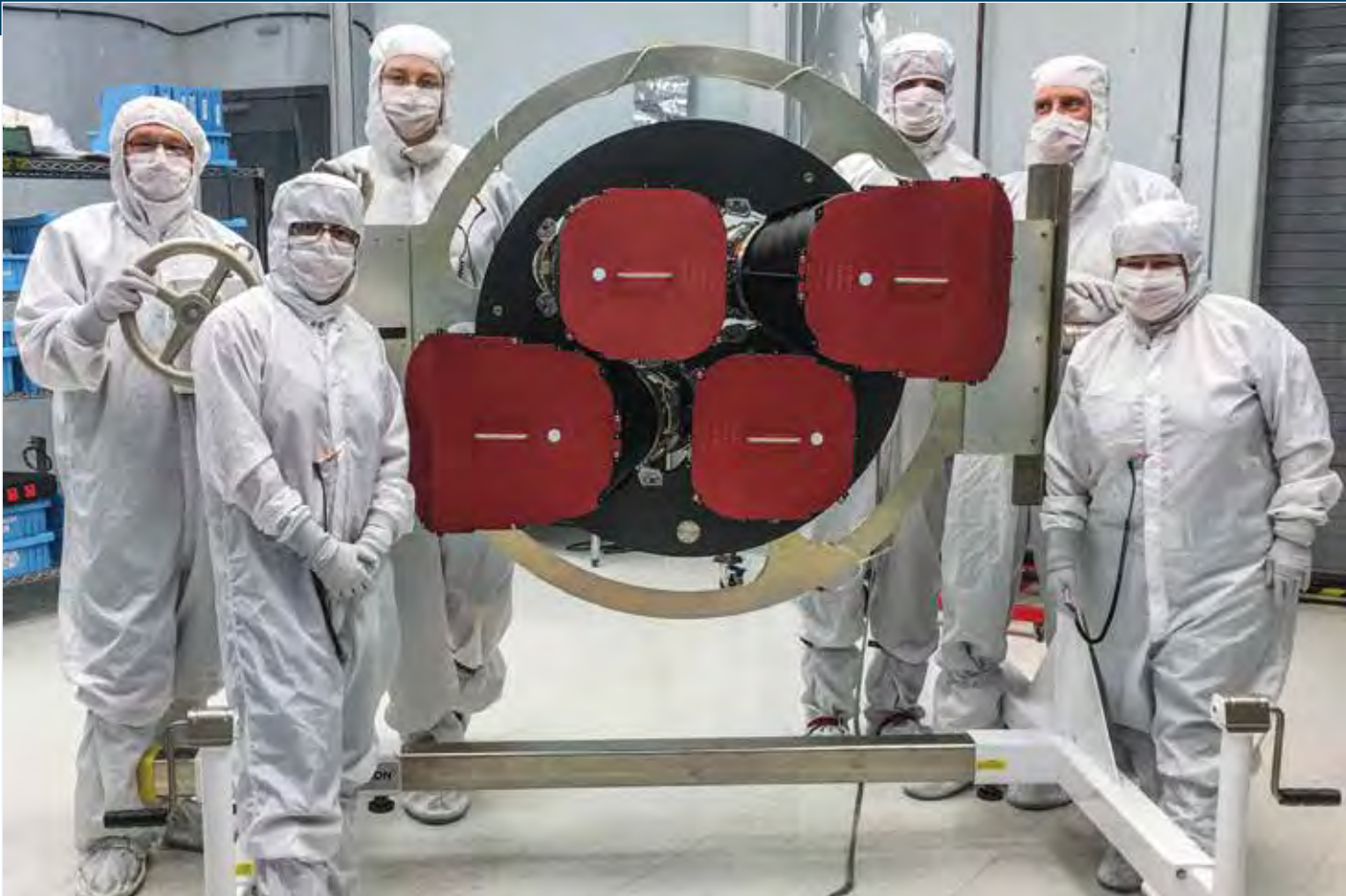
The four TESS flight telescopes with their detector arrays, shown assembled on their base plate, are ready for integration on the spacecraft. Lincoln Laboratory provided the detector arrays, optical subsystem, system engineering, integration and test, and program management for the science payload.
