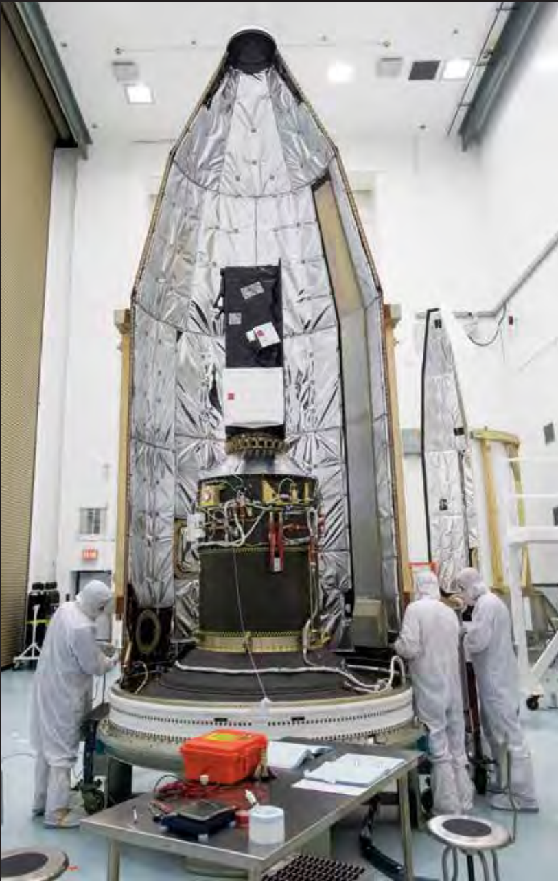
Above, engineers inspect SensorSat prior to thermal-vacuum testing that emulates the conditions the satellite will be exposed to on orbit. Below, in Florida, researchers integrate SensorSat with the Minotaur IV rocket from which it will be deployed into orbit.
