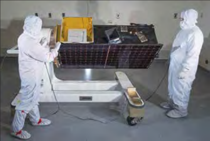
Above, engineers inspect SensorSat prior to thermal-vacuum testing that emulates the conditions the satellite will be exposed to on orbit. Below, in Florida, researchers integrate SensorSat with the Minotaur IV rocket from which it will be deployed into orbit.
