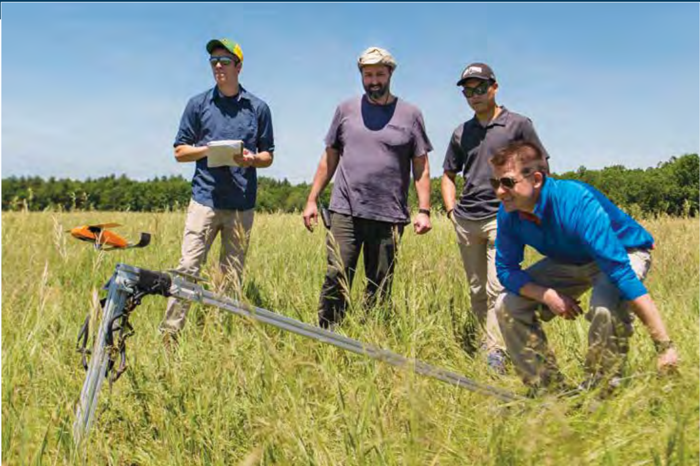
Lincoln Laboratory engineers evaluate flight characteristics of the Perdix micro-unmanned aerial vehicle in various aerodynamic design configurations during a series of ground-launched flight tests on 15 June 2017.
