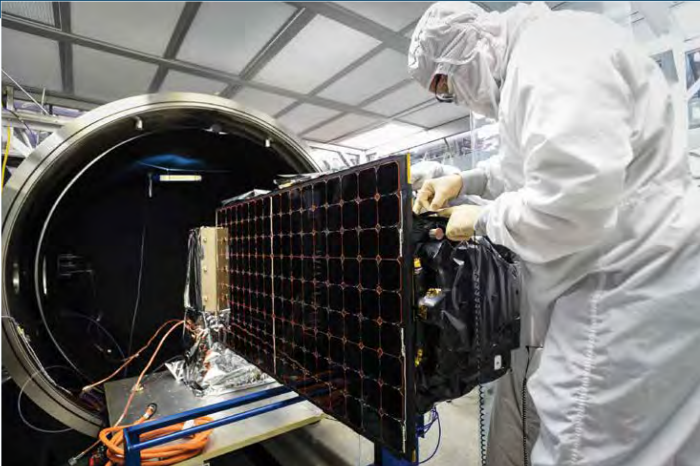
The Operationally Responsive Space-5 SensorSat was delivered to the Air Force after completion of testing to verify the hardware-to-software interfaces, vibration testing to replicate the launch environment, and performance testing in a thermal-vacuum chamber to simulate the space environment.
