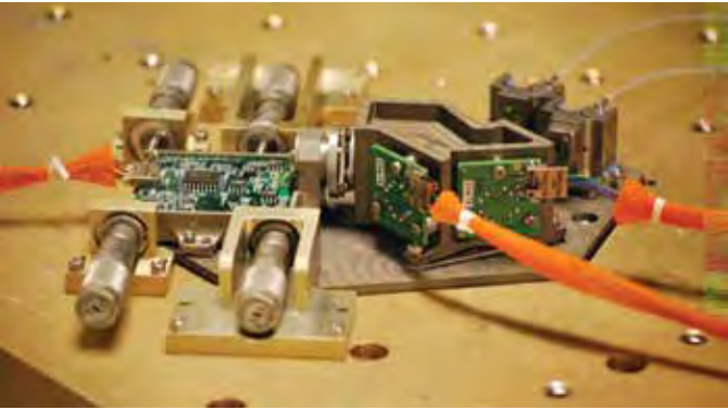
The small optics assembly for the Next-Generation Laser Communications terminal is pictured in the alignment fixture.
