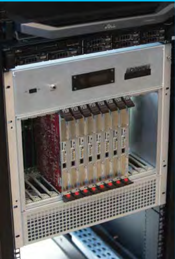
Shown above is a 64-node version of the graph processor. This system has similar processing performance to today's best supercomputers but consumes only 1/100th of the power.
