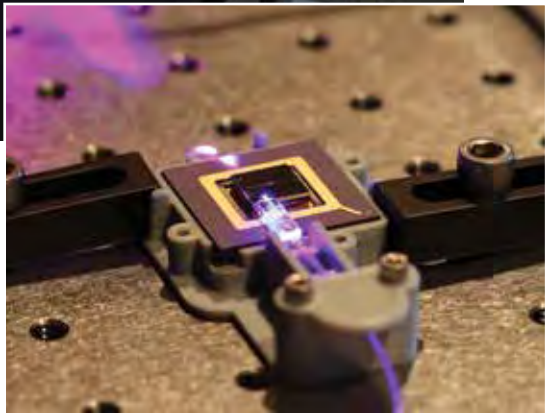
Top, lasers and optics are used to control single-atomic ions. Above, light is sent into an ion trap chip to be routed to the trapped-ion qubit via integrated optics.
