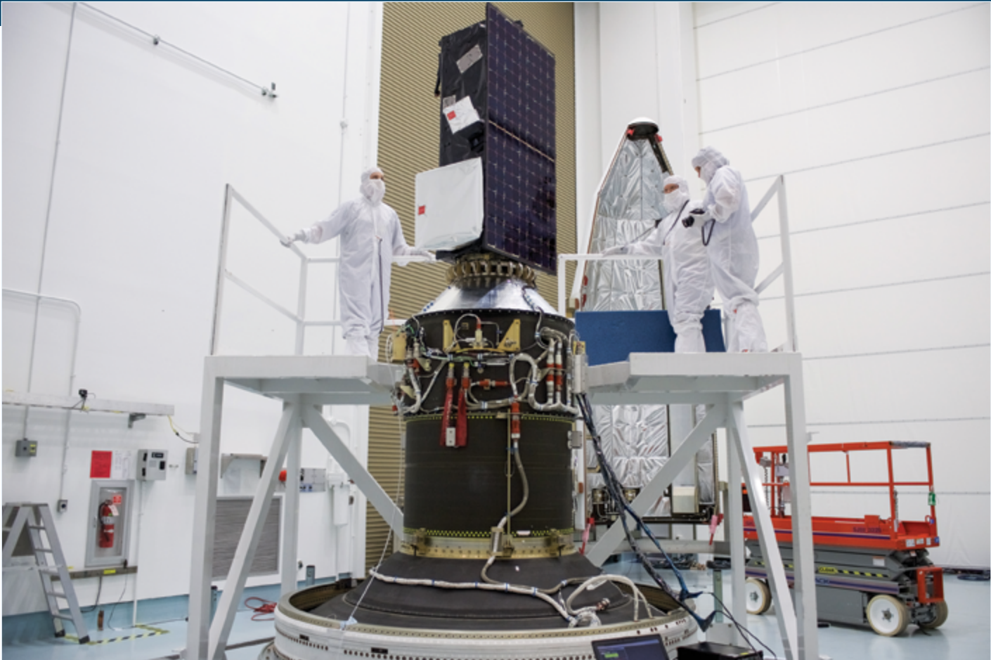
Lincoln Laboratory staff performed the final closeout and inspection of the SensorSat space vehicle during integration on the Minotaur rocket from which it was launched at Cape Canaveral, Florida. SensorSat is now providing data for space situational awareness.
