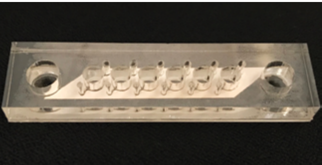
The co-culture system contains six culture wells that can be manipulated directly from the top and the two larger side wells that steadily flow media to the lower chambers via gravity. The upper and lower culture wells are separated by a membrane that allows chemicals to diffuse between the cells above and below to help form physiological tissue.
