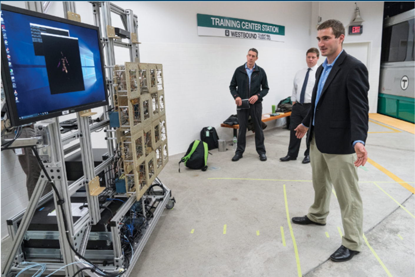
Engineers tested a microwave imaging system in a Massachusetts Bay Transportation Authority training center. The system collects radar reflections off liquid, metal, or plastic objects concealed on pedestrians; algorithms process the imagery in real time to determine if the objects are threat items.
