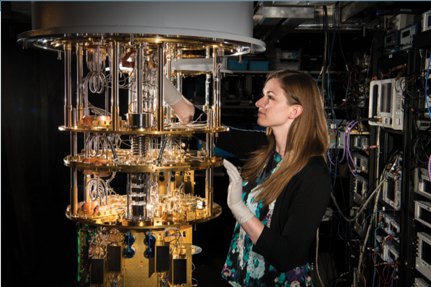
Bethany Huffman adjusts the dilution refrigerator, above, that cools qubit circuits to 20 thousandths of a degree above absolute zero when operating. The Laboratory's 3D approach to fabricating qubits is enabling more flexible and complex circuitry needed to advance superconducting quantum computers.
