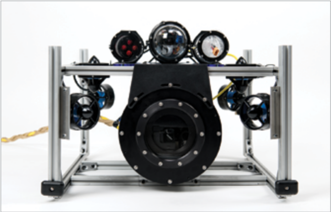
In 2018 tests conducted with this undersea optical communications system in an indoor pool, researchers successfully demonstrated the system's pointing, acquisition, and tracking capabilities.
