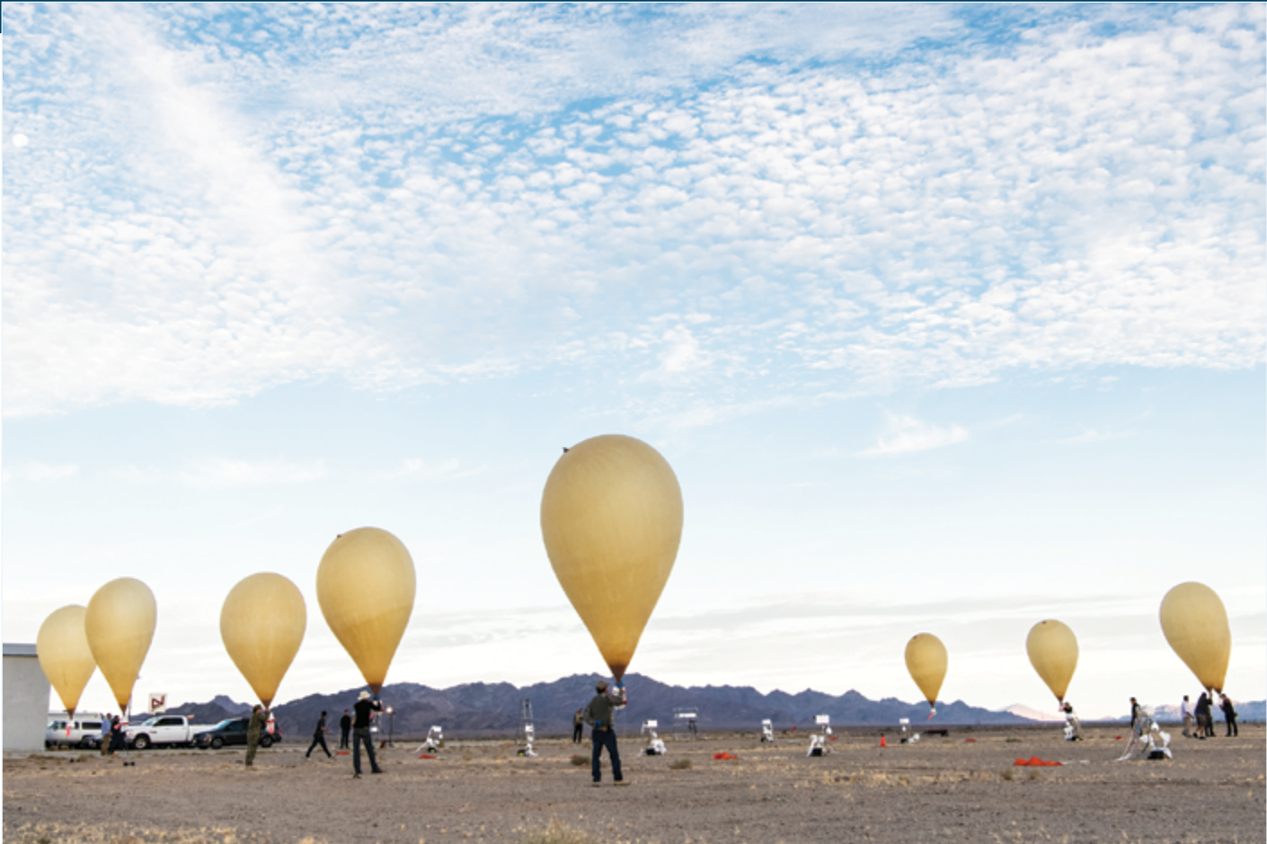
The HALO (High-altitude Attritable Link Offset) program successfully demonstrated the first balloon-based communications relay array. Ten low-cost balloon payloads used distributed adaptive array processing techniques to achieve over-the-horizon communications despite co-channel interference.
