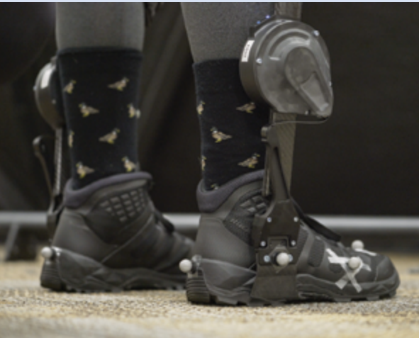
An ankle exoskeleton, like this commercial bionic boot, may help soldiers hike longer and with less stress on muscles.
