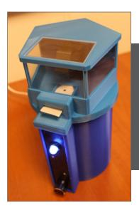
The custom hydrator capable of volatilizing various swabs coated with the Nafion<sup>™</sup> polymer is a cost-effective, 3D-printed device.
