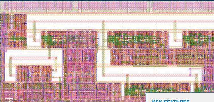
The physical design layout of the "portholes" technique creates "keep-out zones" around a security-critical wire. This approach positions the security-critical components within inspectable regions to make them easier to inspect for malicious modification.
