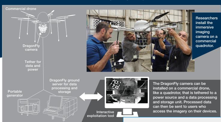
DragonFly, a lightweight, low-power motion imaging system, can be mounted on a mobile platform to capture imagery over a 360-degree horizontal field of view. This system can be rapidly deployed on a tethered drone to provide high-resolution imagery of the area above or below the drone. DragonFly is valuable for monitoring events, areas, or venues, such as outdoor concerts or natural disaster sites, that lack towers, poles, or fences on which stationary cameras can be mounted.
