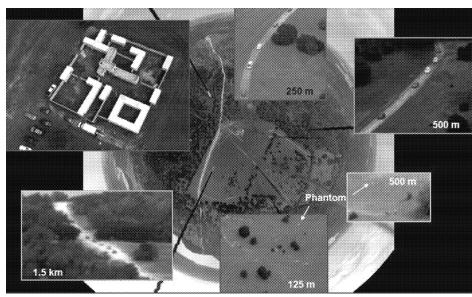
Shown are images captured and processed with DragonFly while its UAV was hovering about 400 feet above a small compound in forested countryside. The camera array used three tiers of cameras each with a different fixed focal length. The ground server stitches together overlapping images to produce a wide-area image of the entire area below the UAV and closeups of any region within that area.
