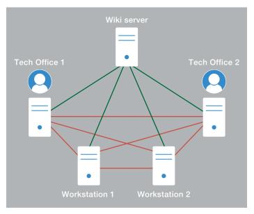
Dynamic Flow Isolation prohibits user access to systems not necessary to the user's work. In this example of a privilege scheme, the workstations may only communicate directly with the wiki server and not each other. This arrangement helps to mitigate attacks that seek to move from one user's workstation to a more privileged workstation like that of a system administrator.
