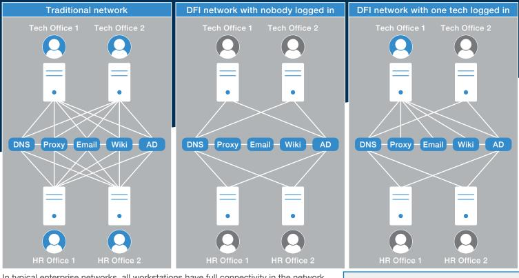
In typical enterprise networks, all workstations have full connectivity in the network layer, potentially allowing attackers unrestricted access to the entire network. In the DFI strategy, systems logged off the network can only access the active directory (AD) and domain name system (DNS), and individuals are restricted to needed services.
