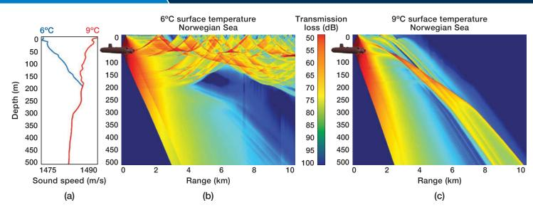
Sound propagation profiles (b and c) generated by a 50-meter-deep sound source can vary drastically depending on variations of temperature across depth (a), which impacts sound speed.
