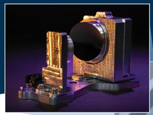
Center, the prototype two-mirror freeform optical design, fabricated via diamond turning, provides a wide field of view and a large aperture.
