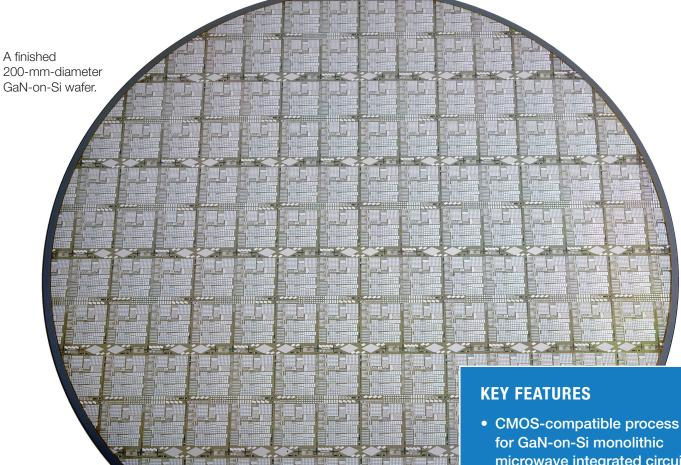
Lincoln Laboratory developed fully Si CMOS-compatible technologies for GaN MMICs on 200-mm-diameter Si wafers. Measured  $\rm f_{T}$  and  $\rm f_{max}$  are in the 50 and 90 GHz range, respectively, for GaN high-electron-mobility transistors (HEMTs) with 120-nm gate length on Si substrates. We are applying wafer-scale 3D integration technology to the heterogeneous integration of GaN MMICs and Si CMOS circuits for high-performance RF modules.
