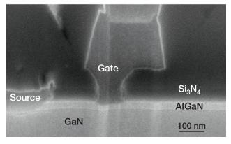
Cross section of a GaN HEMT with sub-100-nm gate length on 200-mm-diameter Si substrate. The fabrication process is fully CMOS compatible, using only optical lithography and gold-free metallization.
