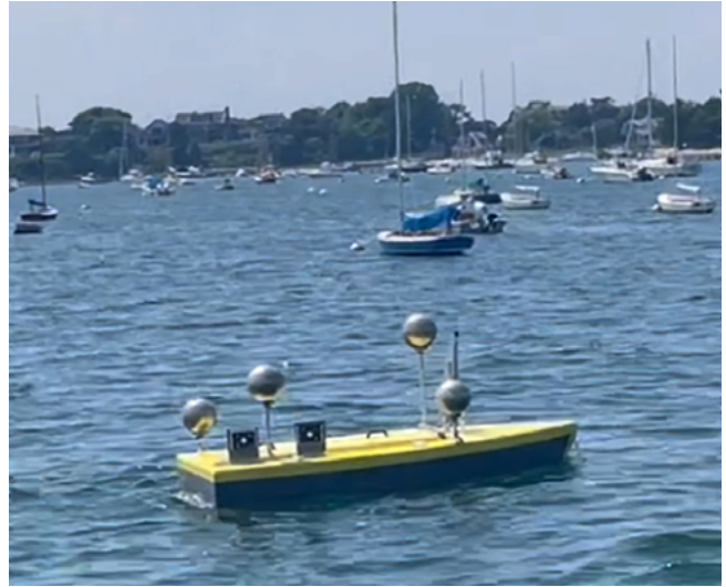
A 12-foot, all-electric prototype ASV with our sonar array mounted underneath was deployed in Woods Hole, Massachusetts, for testing. The full concept calls for an array of ~20 ASVs of about this size, likely powered by wave or solar energy, to map an extensive area.
