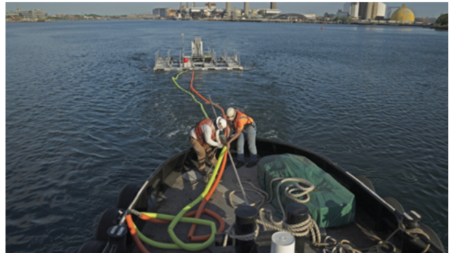
In 2021, researchers deployed a rigid frame on which a technology demonstrator undersea-mapping sparse sonar array was mounted for sea tests of the array's capability intended to provide resolution two orders of magnitude higher than currently achievable.
