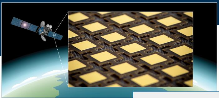
The close-up shows the lower printed circuit board for a lightweight antenna array panel for a space-based radar. The cutouts visible between the elements reduce the panel's weight.
