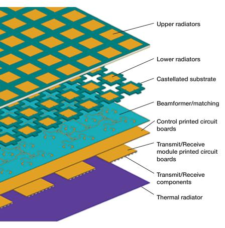
In the exploded view of the layers in the antenna array, the innovation is the castellated substrate. In this layer, material around the lower radiating elements is cut out to reduce the weight of the antenna. These cutouts do not hamper the performance of the antenna.
