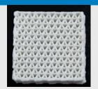
Toluene/isopropanol washing procedure removes residual oil, leaving a fully inorganic part
