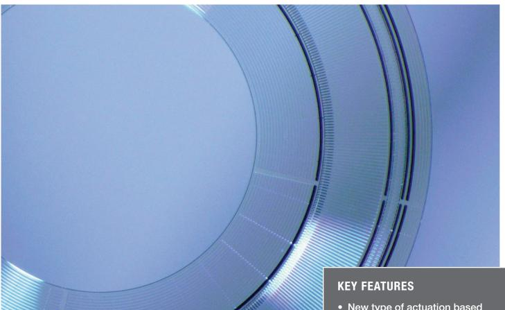
Microhydraulic actuator component suspended on the surface of water.
