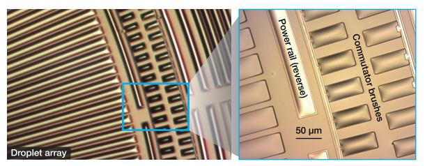
Development of microhydraulic actuators requires microfabrication of thin sheets of material with precisely engineered drops on their surface. Shown here is a 5-µm-thin polyimide sheet with micron-scale water drops. This particular element is a component of a rotational microhydraulic motor (cover photo).
