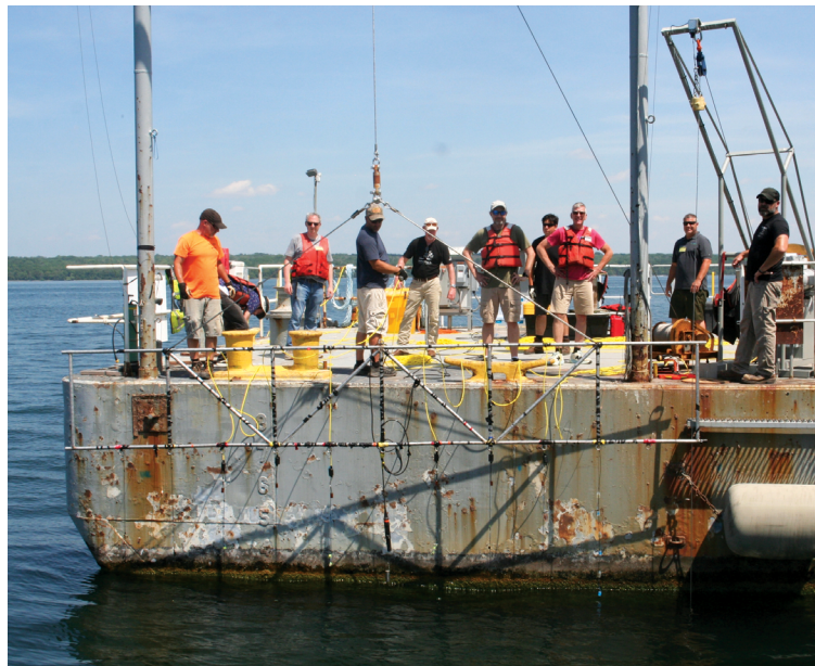
During field tests in 2025, the research team deployed cables with the MEMS hydrophones attached.
