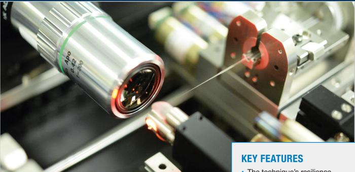
The photonic lantern is fabricated on a high-precision mechanical system. The tip of the photonic lantern is inspected with a microscope objective prior to the lantern's being spliced to a fiber.
