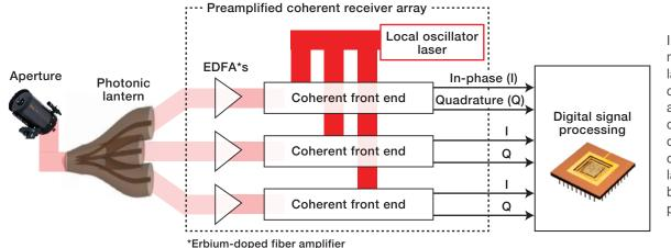
In this overview of a multi-mode photoniclantern receiver concept, signals acquired using parallel coherent detection of the single-mode outputs of the photonic lantern are combined by using digital signal processing.
