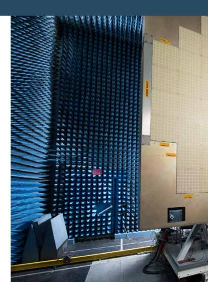
Multifunction Phased Array Radar (MPAR) System in the RFSTF Large Near-Field Scanner Facility
