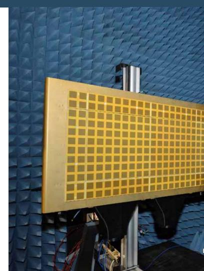
MPAR Panels Under Test in the Small Near-Field Scanner Chamber
