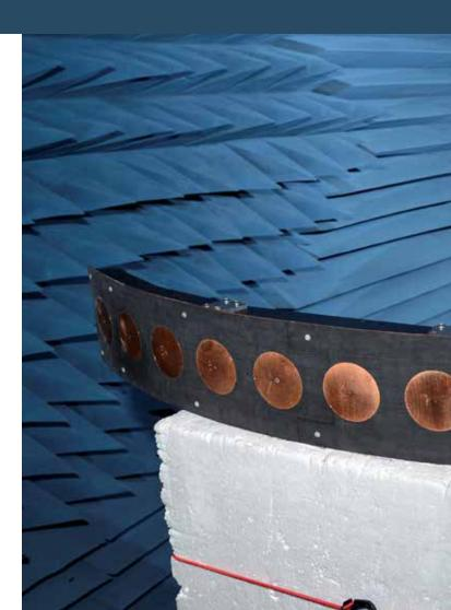
3D-Printed Copper-Plated Conformal Array Under Test in the Tapered Chamber
