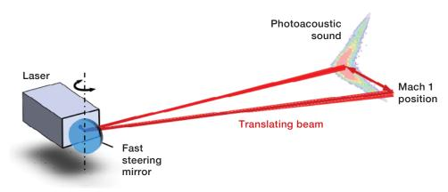
The TALC system uses a fast steering mirror to control the sweep speed of a laser beam (translating beam). The two beams directed from the fast steering mirror represent the laser beam at two different times (i.e., mirror positions). When the beam sweep speed matches the speed of sound (Mach 1), a strong audio signal is produced. This Mach 1 condition only occurs at a particular range, thus a strong photoacoustic signal occurs only at this range.
