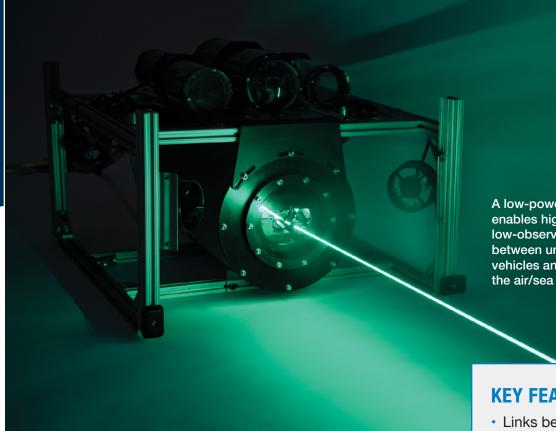
A low-power laser beam enables high-speed, low-observable links between undersea vehicles and through the air/sea interface.
