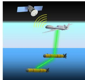
Above, optical communication between undersea terminals is supported up to 400 meters, depending on water clarity. At left, optical communication enables real-time, highspeed communication between underwater devices, airborne vehicles, and beyond.
