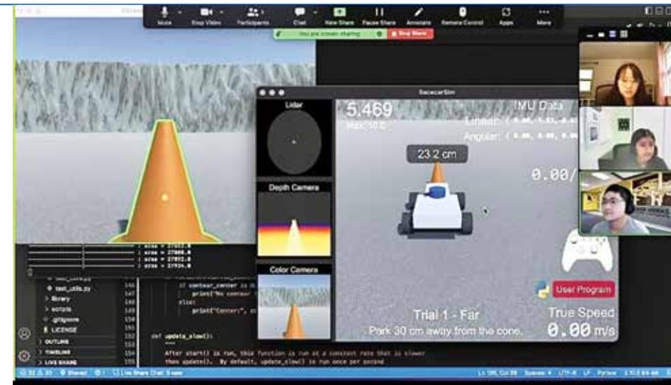
Students in the RACECAR course learn how to train an autonomous vehicle to follow colored lines using color priority swapping through a queue. The racecar is able to automatically turn to follow a colored line on the ground and can be directed to drive toward multiple final destinations given the state of the car.
