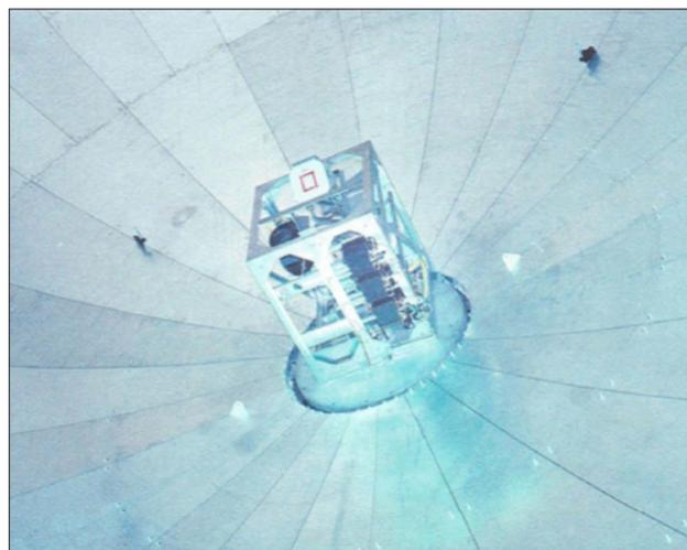
**FIGURE 11.** The MMW optical beam waveguide is shown being tested in the anechoic chamber at Lincoln Laboratory (left) and after installation on the radar (right).
