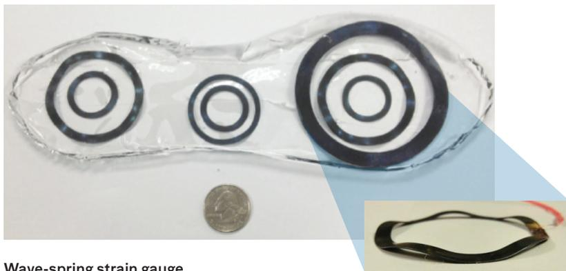
Wave-spring strain gauge.
