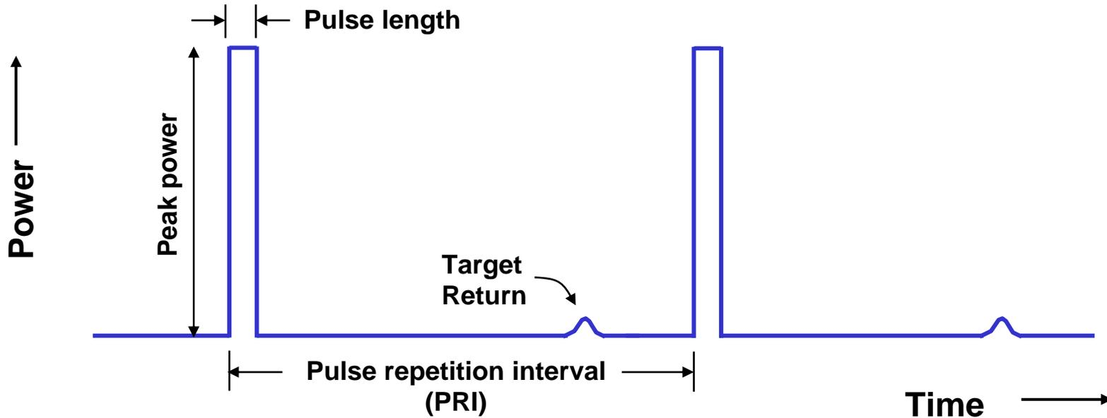
$$\text{Duty cycle} = \frac{\text{Pulse length}}{\text{Pulse repetition interval}}$$
