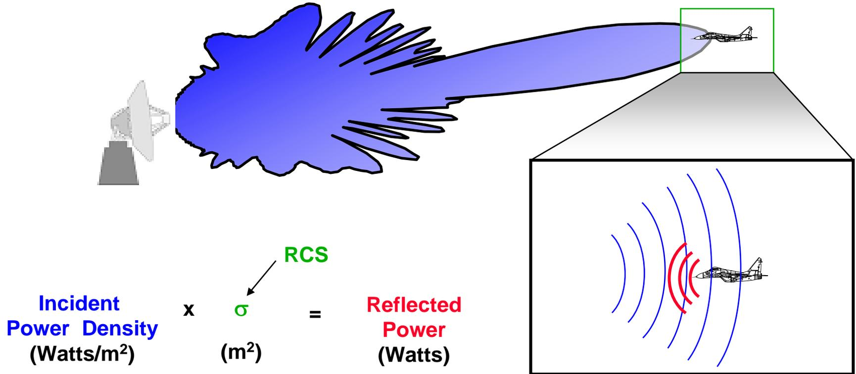
Radar Cross Section (RCS, or  $\sigma$ ) is the effective cross-sectional area of the target as seen by the radar
