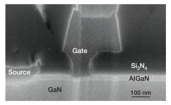
Cross section of a GaN HEMT with sub-100-nm gate length on 200-mm-diameter Si substrate. The fabrication process is fully CMOS compatible, using only optical lithography and gold-free metallization.
