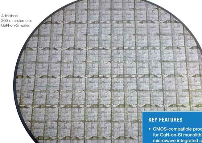
Lincoln Laboratory developed fully Si CMOS-compatible technologies for GaN MMICs on 200-mm-diameter Si wafers. Measured  $\rm f_{T}$  and  $\rm f_{max}$  are in the 50 and 90 GHz range, respectively, for GaN high-electron-mobility transistors (HEMTs) with 120-nm gate length on Si substrates. We are applying wafer-scale 3D integration technology to the heterogeneous integration of GaN MMICs and Si CMOS circuits for high-performance RF modules.
