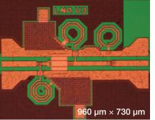
Example of an X-band low-noise amplifier that delivers 10 dB of gain. The GaN-on-Si MMIC process adds metal-insulator-metal capacitors, metal resistors, inductors, and two levels of thick interconnect metals.
