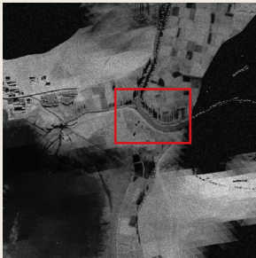
Step 3 If vehicles are identified in GMTI data, analyst requests synthetic aperture radar (SAR) imagery for more focused view of vehicles.
