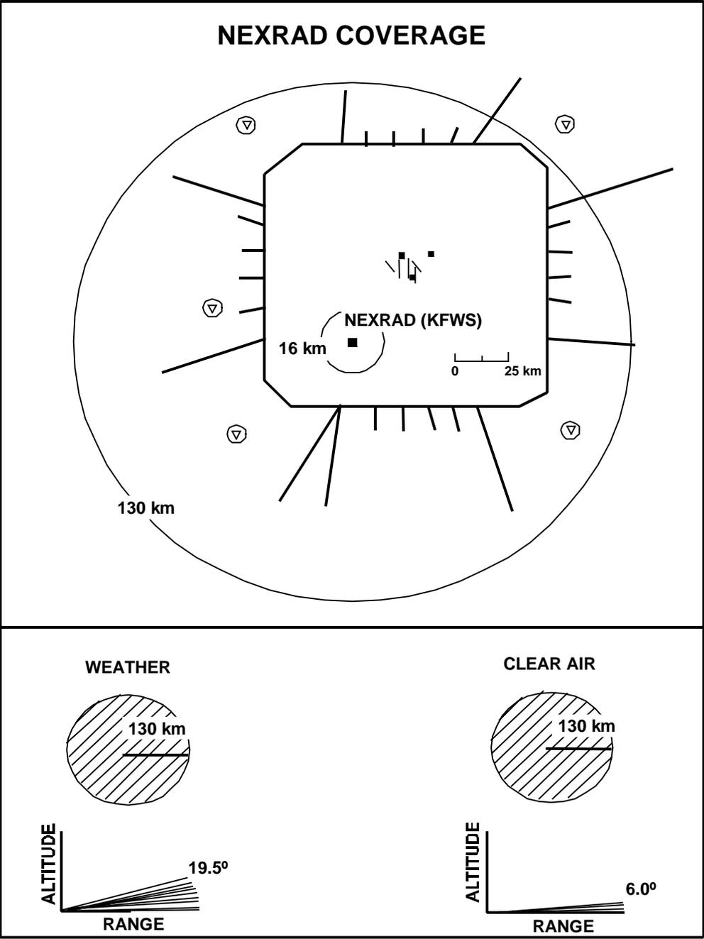
Figure 6. KFWS NEXRAD location and coverage region. In this study, reflectivity data were used for the regions between 16 km and 130 km from the radar. Data closer than 16 km were not used because the data in that region do not extend to an altitude of at least 6 km. The lower Figure shows a plan view of the scanning range and a vertical cross section of the scan strategy for both "weather" and "clear-air" modes.
