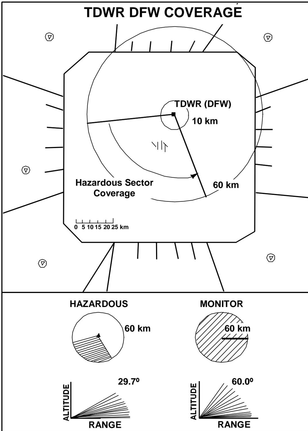
Figure 8. The location and coverage region for the DFW TDWR. Data were used beyond 10km and within 60 km of the radar. The lower Figure shows a plan view of the scanning range and a vertical cross section of the scan strategy for the radar in "hazardous" and "monitor" modes.
