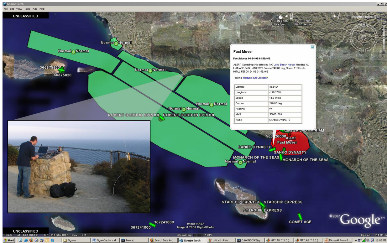
FIGURE 8. During a field data collection from Point Dume State Beach in Malibu, Calif., in June 2008, the FET recorded and ingested data from the maritime Automatic Identification System (AIS). One of the ships (the Sanko Dynasty ) was detected as a fast mover, with a speed faster than the normal speed of maritime traffic in Long Beach Harbor. This alert caused a warning state to be activated, indicated by the Long Beach Harbor watchbox (shaded red), alerting the user to abnormal activity in that area.
