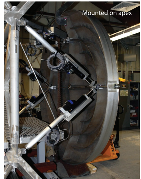
FIGURE 7. The subreflector is a 112-inch (2.8 m)-diameter hyperboloid. It was fabricated from an aluminum casting that was subsequently machined to a 32 \mu\text{m} rms surface accuracy. The subreflector is mounted near the apex of the quadrapod on six actuators that permit displacement and rotation of the subreflector along three orthogonal axes.
