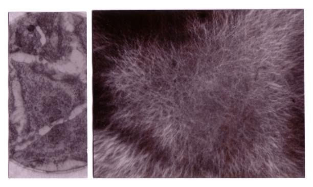
This comparison of micrographs of a cell shows the higher resolution made possible by the solid-immersion lens (right) over conventional microscopy (left). Both images were made using identical microscope objectives and magnifications. The cell is about 40 micrometers across.
