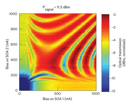
The color-coded map shows constructive and destructive interference as a function of bias current on the two semiconductor optical amplifiers (SOA 1 and SOA 2). Constructive interference between the two interfering light beams, shown in deep red, results in high optical transmission (a digital 1), while destructive interference, shown in blue, produces low optical transmission (a digital O).
