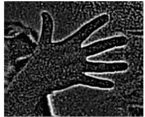
Figure 2. On-chip spatial linear filtering produces an edge detection image.
