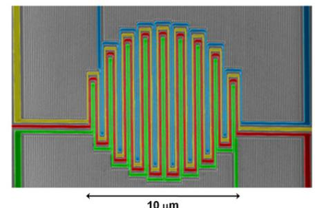
Figure 1. (a) A schematic of a single SNPD. The nanowire is typically 4 nm to 6 nm thick and 50 nm to 100 nm in width. (b) A false-color scanning electron micrograph of a four-element SNPD array.
