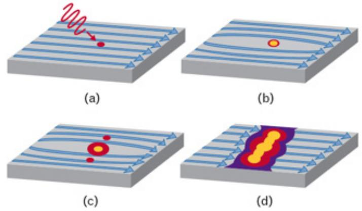
Figure 2. (a) An incident photon heats a nanowire, forming a localized hot spot (b) where the superconductivity is disrupted. The supercurrent diverts around this spot. (c) When the local current density on either side of the hot spot exceeds the critical current density, a resistive region spanning the entire cross section of the nanowire is formed (d).
