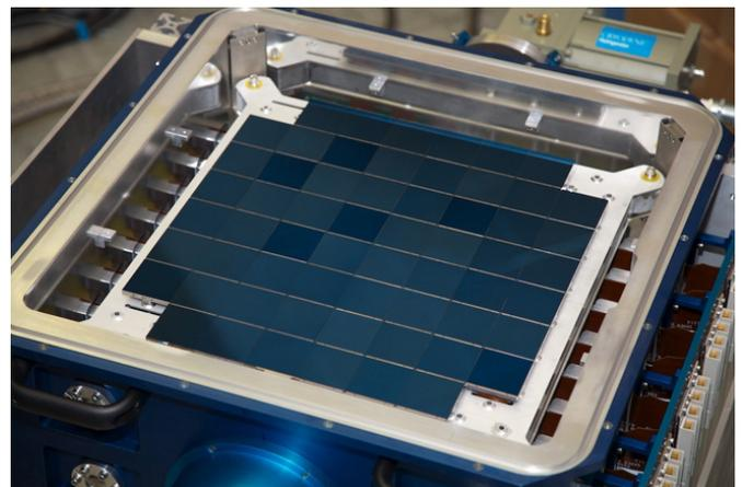
The Pan-STARRS focal plane array contains 60 orthogonal transfer arrays, comprising about 1.4 billion pixels in the 16 in<sup>2</sup> area. Photograph courtesy of John Tonry, University of Hawaii.
